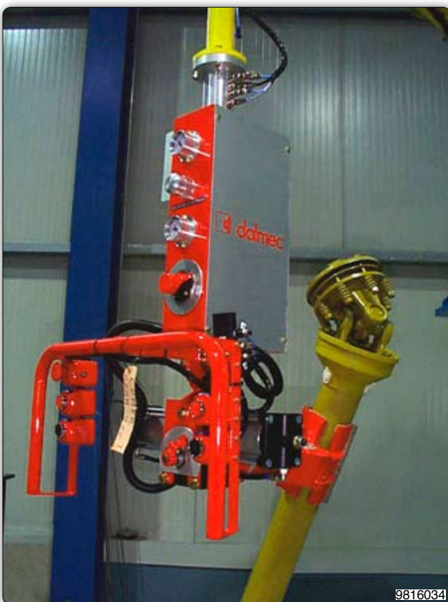
Manipulator with pneumatic tooling for gripping and rotation of transmission shafts. 装备气动工具的机械手臂，可抓取和旋转传动轴。
