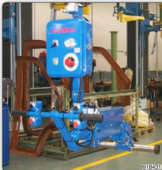
Manipulator with pneumatic tooling for gripping and inclination of shafts. 装备气动工具的机械手臂，可抓取和倾斜传动轴。
