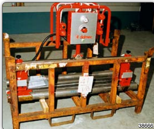
Manipulator with double gripping head tooling for gripping and handling transmission shafts. 装备双抓取头的机械手臂，可抓取和搬运传动轴。
