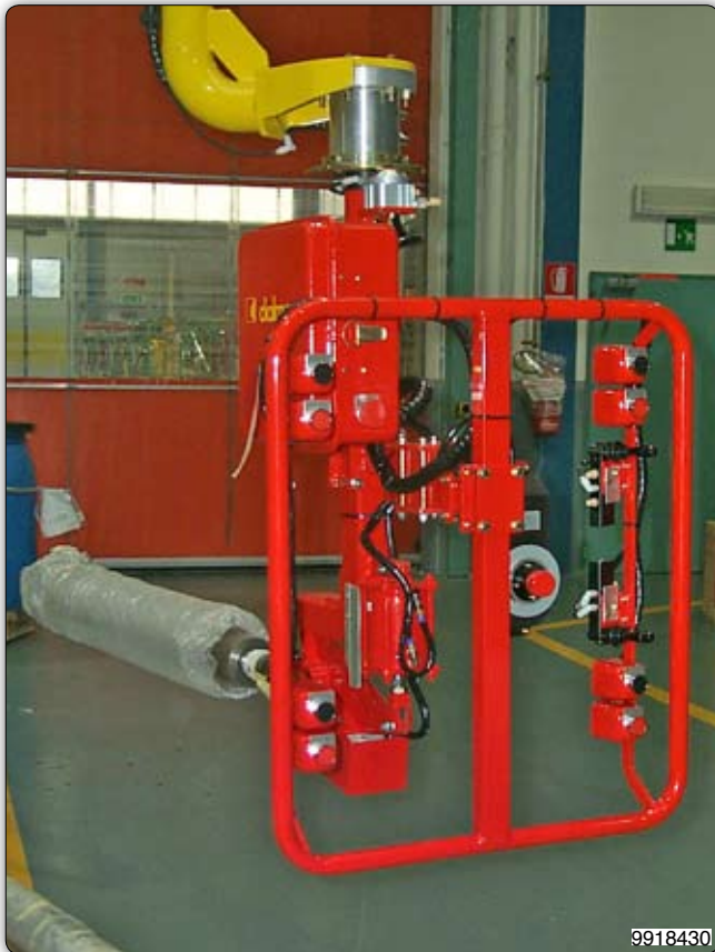
Manipulator with pneumatic tooling for gripping and handling shafts. 装备气动工具的机械手臂，可抓取和搬运传动轴。
