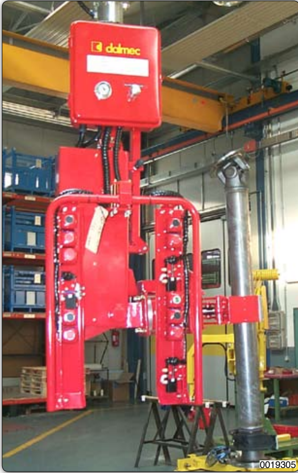
Manipulator with jaws tooling for gripping and rotation of transmission shafts.
