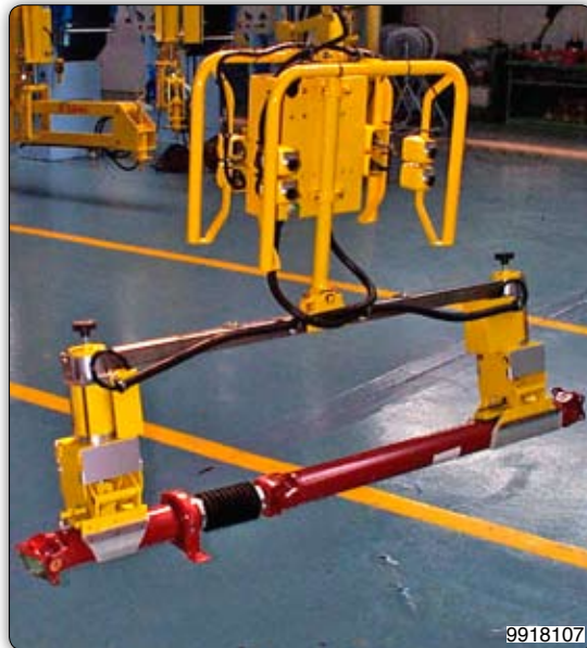
Manipulator with adjustable jaws and double gripping head tooling for handling transmission shafts. 装备可调整卡爪和双抓取头的机械手臂，可搬运传动轴。
