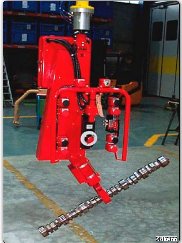
Manipulator with pneumatic tooling for gripping and inclination of mechanical shafts.
