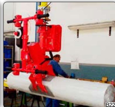
Manipulator with pneumatic gripping jaws for the easy picking of stacked reels about their external diameter. Manipulator 装备气动卡爪，可以从外径轻松抓取包装卷轴
