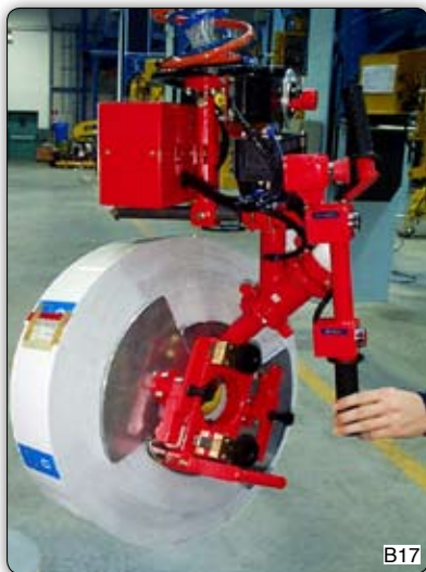
Manipulator with "Venturi" suction cups tooling for gripping reels, with manual rotation from horizontal to vertical. Manipulator 配备文丘里真空吸盘，抓取卷轴，可以从横向到纵向手动翻转
