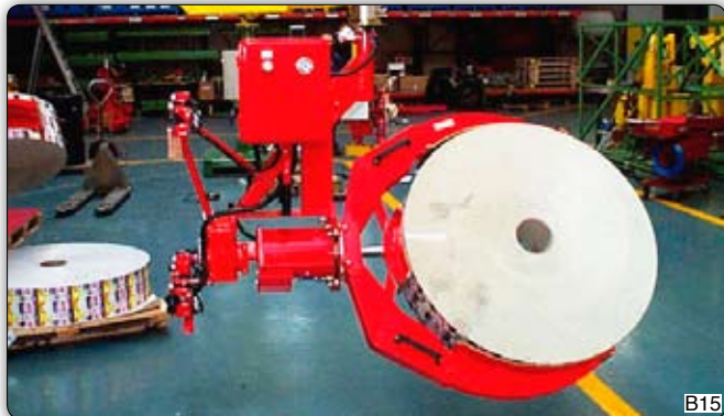
Manipulators fitted with gripper tooling for handling reels about their outside diameter, with pneumatic 360° rotation.
