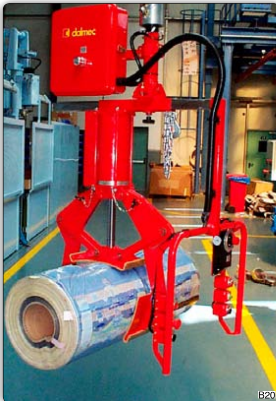
Manipulator fitted with pneumatic grippers for handling reels about their outside diameter. Manipulator 可从卷轴外径气动抓取。
