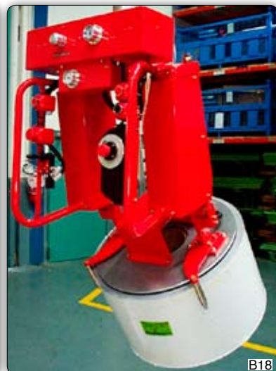
Manipulator with "Venturi" vacuum suction ring and 90° pneumatic inclination. Manipulator 配备文丘里真空吸盘，可90度气动倾斜。
