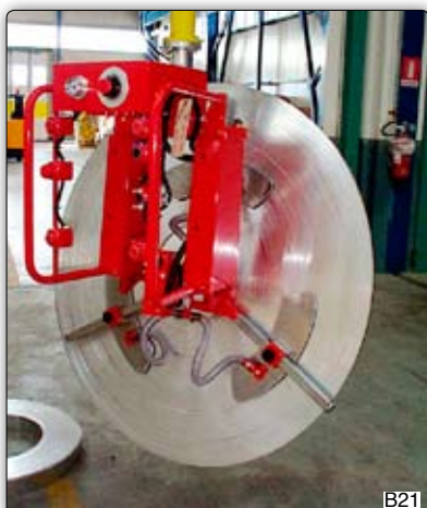
Manipulator with manually adjustable suction cups tooling for gripping and 90° inclination of rolls of metallic banding. Manipulator 可手动调节吸附盘，可以抓取和90度倾斜带有金属箍的球。
