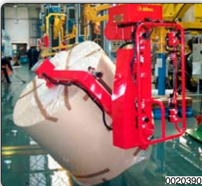
Expanding mandrel for the pneumatic rotation of reels. 涨开式心轴，用于气动转动卷轴。
