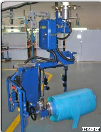
Manipulator with expanding mandrel for picking, inclination and manual rotation of reels. Manipulator 配备涨开式心轴，可抓取，倾斜和气动翻转卷轴。
