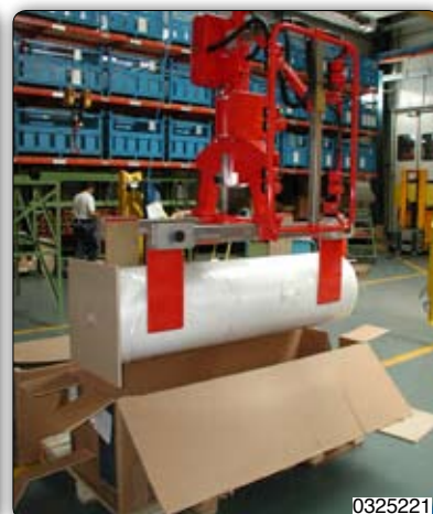
Adjustable jaws tooling for handling reels and their packaging. 可调卡爪，用于搬运卷轴及其包装。
