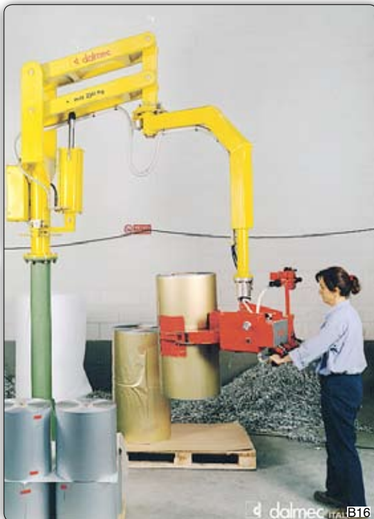
PMC type Partner manipulator, column mounted, with gripper tooling, for handling reels about their external diameter, with pneumatically assisted rotation through +/- 90°. Manipulator (partner PMC 支柱式，配备可抓取卷轴外径的抓取工具，可+/-90度旋转。
