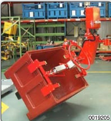
Partner PMC column mounted with pneumatic tooling for gripping, inclination and manual rotation of plastic containers having different dimensions. Partner PMC, 支柱式, 装备气动工具, 用于抓取, 倾斜和手动翻转不同尺寸的塑料容器。
