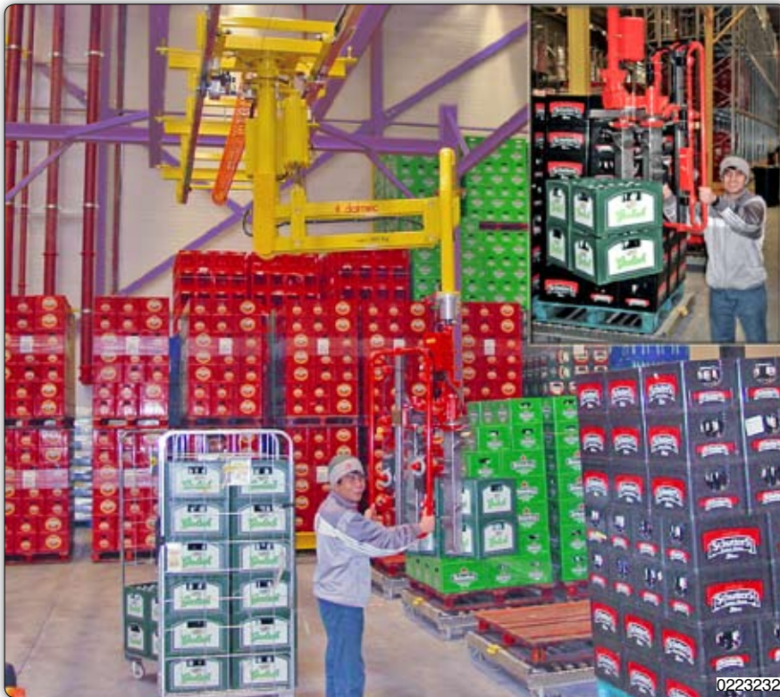
Partner Manipulator overhead trolley mounted version with pneumatic motorization, equipped with multiple adjustable hooks gripping system for handling 1 to 8 beverage crates having different dimensions. Manipulator Partner, 高架行车式, 装备气动马达, 多个型号挂钩, 可以搬运1到8个尺寸不同的饮料包装箱。
