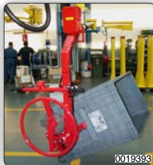
Gripping devices for handling containers of food products. In particular: 用于抓取食品容器的抓取工具。如下: - jaws tooling suitable for gripping and emptying carton boxes, containing tobacco, having different dimensions -卡爪, 适用于抓取和倒空装有烟草的不同大小的纸箱。 - a simple tooling for plastic boxes with manual rotation 可以手动翻转的用于抓取塑料盒子的简单工具。 - hooks tooling made of stainless steel for handling plastic boxes 由不锈钢制成用于抓取塑料盒子的挂钩。 - jaws stainless steel tooling for handling plastics boxes containing apples. 由不锈钢制成的卡爪, 用于抓取装有苹果的塑料盒子。
