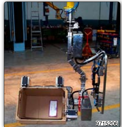
Manipulator provided with jaws tooling made of stainless steel to pick and turn cases. 装备有不锈钢制成的卡爪的机械手臂, 用于抓起和翻转箱子。
