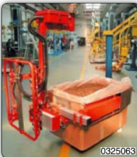
Gripping devices for handling containers of food products. In particular: 用于抓取食品容器的抓取工具。如下: - jaws tooling suitable for gripping and emptying carton boxes, containing tobacco, having different dimensions -卡爪, 适用于抓取和倒空装有烟草的不同大小的纸箱。 - a simple tooling for plastic boxes with manual rotation 可以手动翻转的用于抓取塑料盒子的简单工具。 - hooks tooling made of stainless steel for handling plastic boxes 由不锈钢制成用于抓取塑料盒子的挂钩。 - jaws stainless steel tooling for handling plastics boxes containing apples. 由不锈钢制成的卡爪, 用于抓取装有苹果的塑料盒子。
