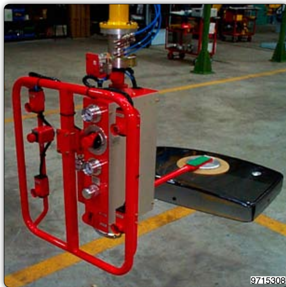
Manipulator with suction cups tooling for gripping and 90° inclination of glasses for TV tubes. Manipulator装备吸盘，用于抓取和90度倾斜应用到电视机显像管上的玻璃。
