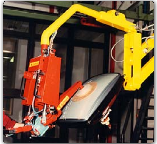
Manipulators with suction cup tooling (Venturi) for gripping, inclination and rotation of TV tubes. Manipulators 装备文丘里吸盘，用于抓取倾斜和旋转电视机显像管。
