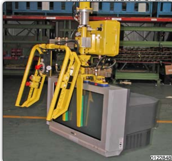
Manipulator with suction cups tooling for gripping on the screen, handling and placing into the appropriate TV packing. Manipulator 装备吸盘，用于抓取显示屏幕，并将其放在组装电视的合适位置上。
