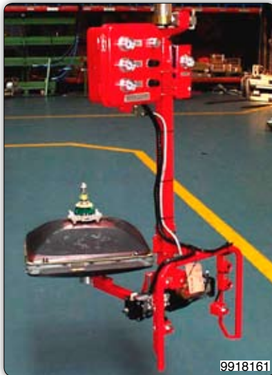
Manipulator with suction cup tooling (Venturi) for gripping and 180° pneumatic overturning of TV tubes and the suction cup is manually rotating. Manipulator 装备文丘里吸盘，用于抓取和气动倾斜电视机显像管，吸盘可手动旋转。
