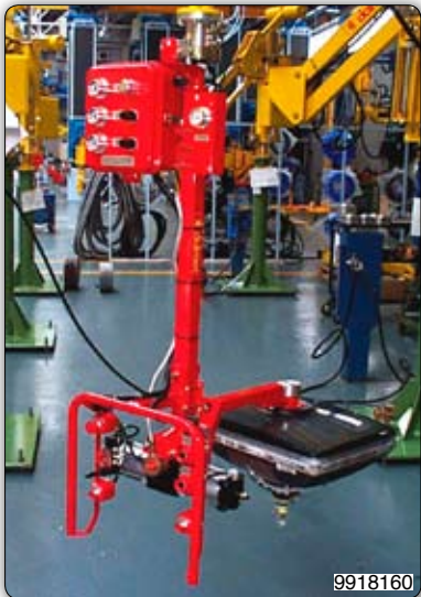
Manipulator with suction cup tooling (Venturi) for gripping and 180° pneumatic overturning of TV tubes and the suction cup is manually rotating. Manipulator 装备文丘里吸盘，用于抓取和气动倾斜电视机显像管，吸盘可手动旋转。
