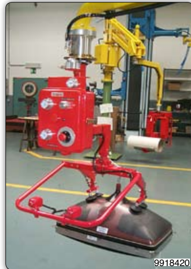
Manipulator with suction cups tooling (Venturi) for gripping and handling of TV tubes on the cone. Manipulator 装备文丘里吸盘，用于抓取倾斜和旋转电视机显像管。
