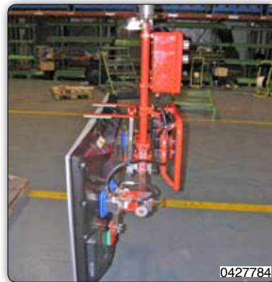
Manipulator with suction cups tooling for gripping and handling TV LCD. Manipulator装备吸盘，用于抓取和搬运电视机LCD。
