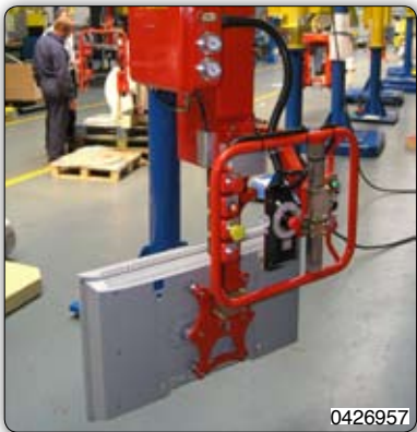
Manipulator with suction cups tooling for gripping and handling TV LCD. Manipulator装备吸盘，用于抓取和搬运电视机LCD。
