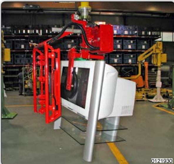
Manipulator with suction cups tooling for gripping and handling TV. Manipulator 装备吸盘，用于抓取和搬运电视机。
