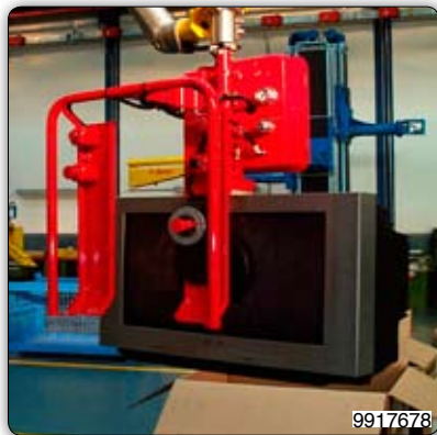
Manipulator with suction cups tooling for gripping and handling TV. Manipulator装备吸盘，用于抓取和搬运电视机。
