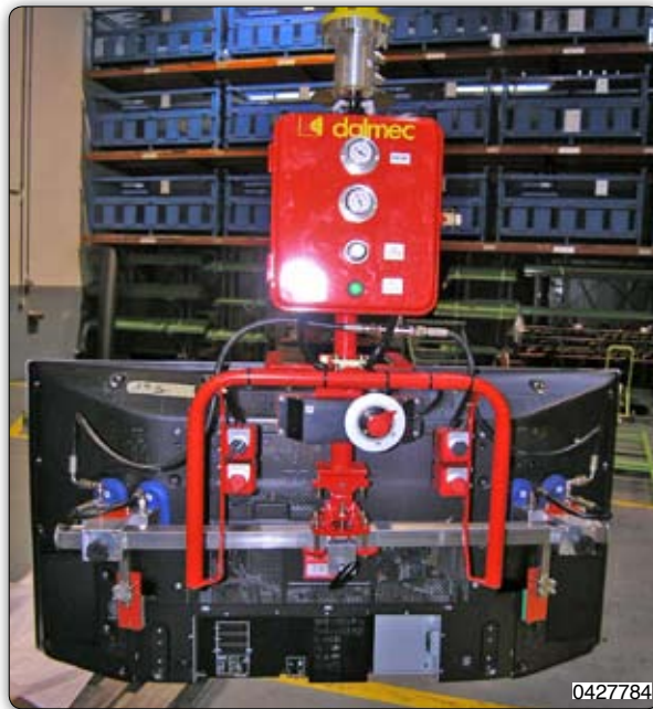
Manipulator with suction cups tooling for gripping and handling TV LCD. Manipulator装备吸盘，用于抓取和搬运电视机LCD。
