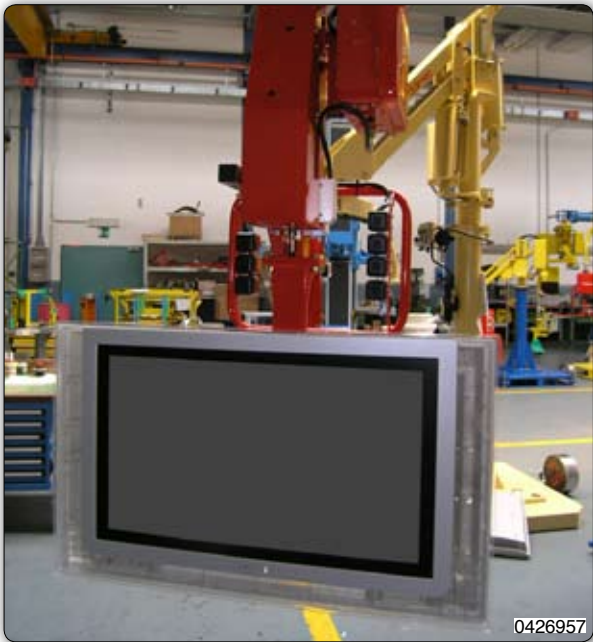
Manipulator with suction cups tooling for gripping and handling TV LCD. Manipulator装备吸盘，用于抓取和搬运电视机LCD。
