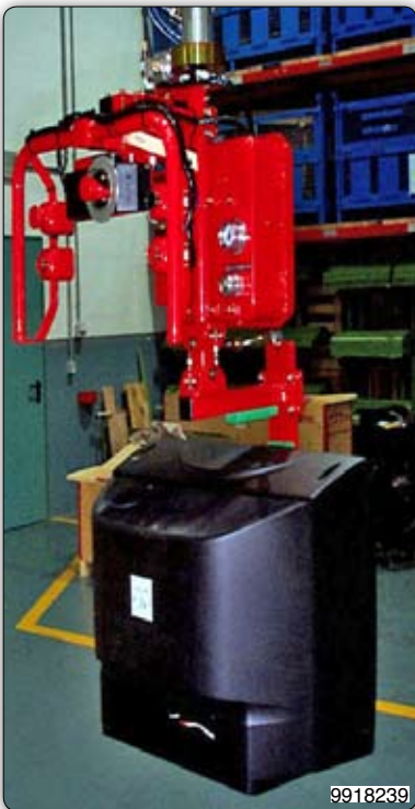
Manipulator with suction cups tooling for gripping on the screen, handling and placing into the appropriate TV packing. Manipulator 装备吸盘，用于抓取显示屏幕，并将其放在组装电视的合适位置上。
