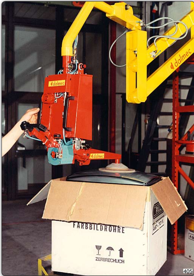
Manipulators with suction cup tooling (Venturi) for gripping, inclination and rotation of TV tubes. Manipulators 装备文丘里吸盘，用于抓取倾斜和旋转电视机显像管。
