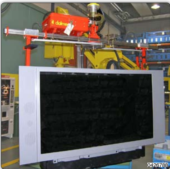
Manipulator with suction cups tooling for gripping and handling TV LCD. Manipulator装备吸盘，用于抓取和搬运电视机LCD。
