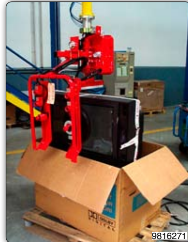
Manipulator with suction cups tooling for gripping on the screen, handling and placing into the appropriate TV packing. Manipulator 装备吸盘，用于抓取显示屏幕，并将其放在组装电视的合适位置上。
