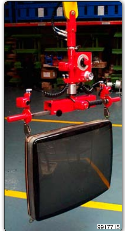
Manipulator with adjustable hooks tooling for gripping the TV tube on the supports. Manipulator 装备可调整挂钩，用于抓取电视机显像管。
