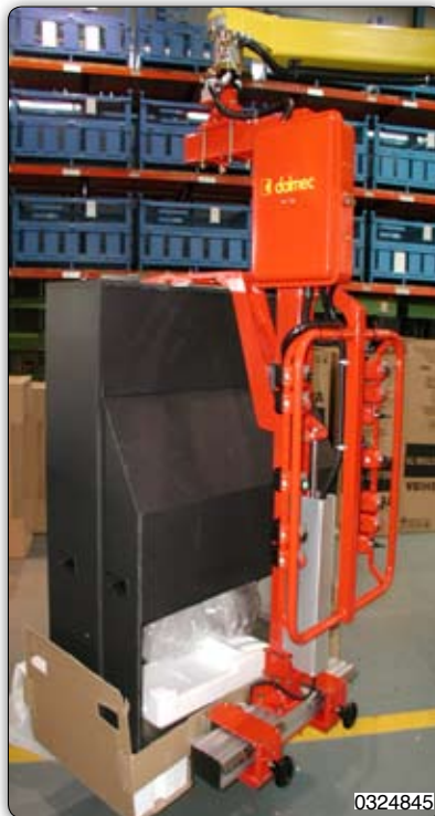
Manipulator with forks tooling for handling packaged televisions. Manipulator 装备叉，用于搬运以组装好的电视。
