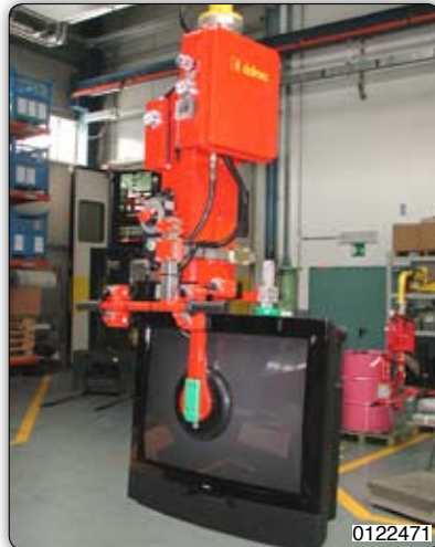
Manipulator with suction cups tooling for gripping and handling TV. Manipulator 装备吸盘，用于抓取和搬运电视机。
