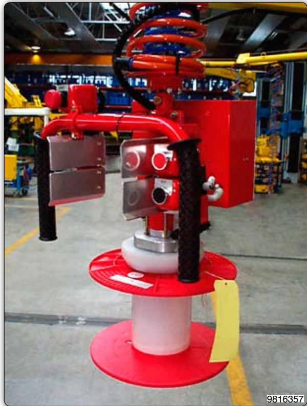
Manipulator with expanding mandrel for picking coils via the core. 通过膨胀心轴抓取线圈的机械手臂。
