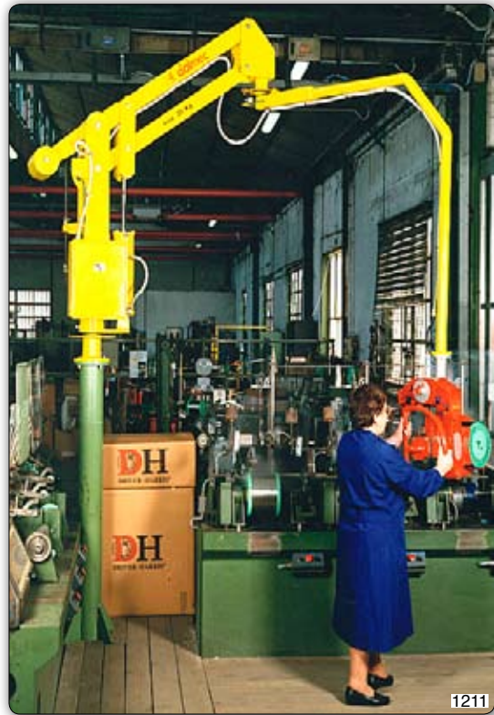
PMC type Partner manipulator, column mounted, provided with gripper tooling to pick metal coils on their central belt. Manipulator Partner PMC, 支柱式，通过线圈中心带来抓取金属线圈。
