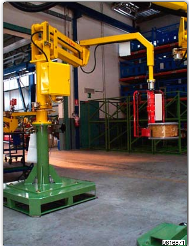
PMC type Partner manipulator, column mounted, fitted with pneumatic action gripper tooling for picking coils of wire on the central belt. Manipulator Partner PMC, 支柱式, 装备气动抓手, 通过中央带抓取线圈。
