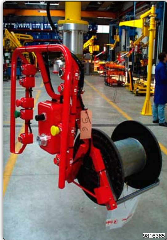
Manipulator fitted with fork-type for handling coils via the flange. Part-present sensors are fitted to the head. 装备叉形头的机械手臂，通过抓取法兰而抓取线圈。工具头中部分安装感应器。
