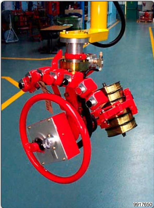
Manipulator with pneumatic jaws for picking multiple coils, with manual rotation of 90°. 装备气动抓手的机械手臂，可抓取多个线圈，可手动旋转90度。
