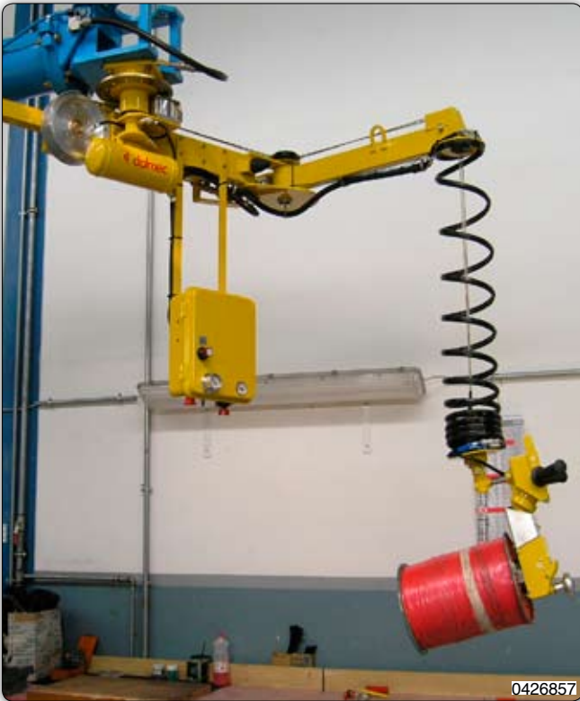
SPF type Speedyfil manipulator, fixed overhead tooling model, fitted with special tooling for picking via an expanding mandrel gripping in the core and manual inclination at 90°. The tooling design caters for automatic picking and release of the coil. Manipulator Speedyfil SPF, 墙式，通过膨胀轴抓取线卷的中心并翻转。这套工具为迎合自动抓取和释放线卷而设计。
