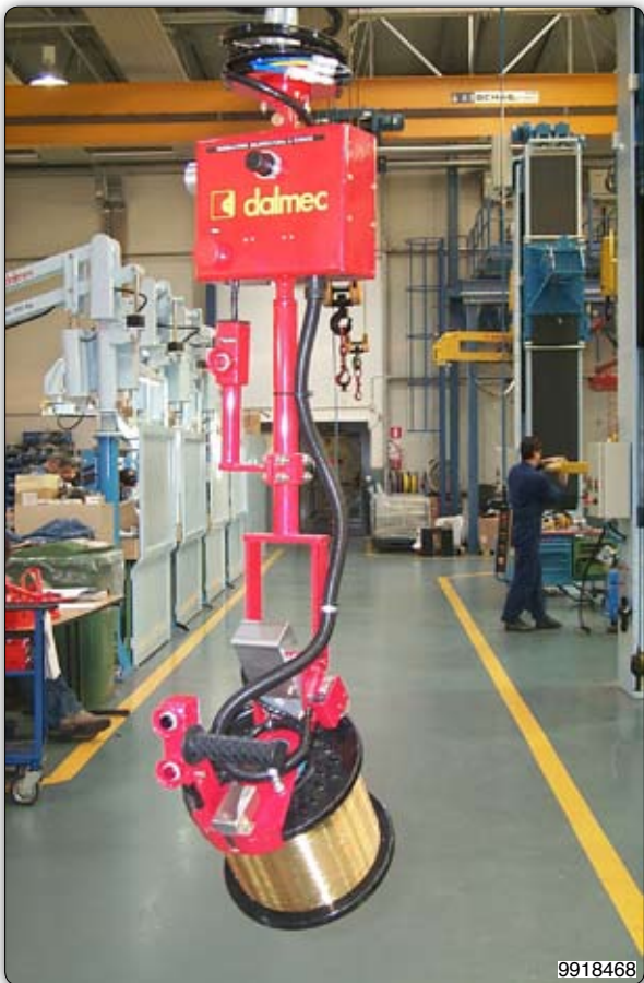
Manipulator designed to pick on the coil's flange with pneumatically actuated tooth, with manual inclination of the coil from the vertical axis to 60 degrees. 通过气动抓手抓取线圈的机械手臂，可纵向60度手动旋转线圈。
