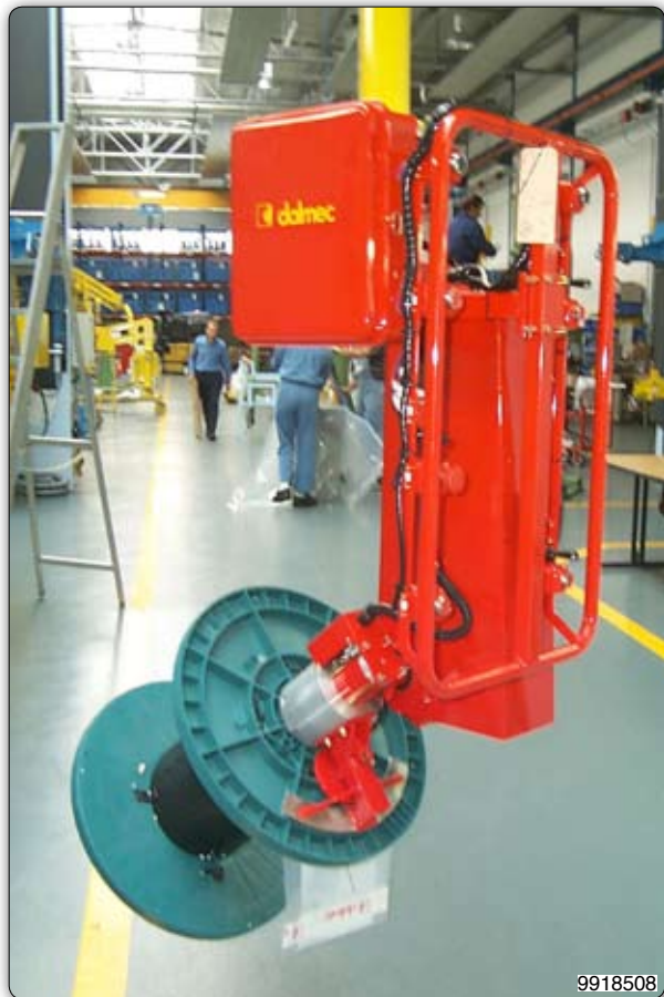
Manipulator with expanding mandrel for picking coils via the cores, with pneumatic 90° inclination. 通过膨胀心轴抓取线圈的机械手臂，可气动倾斜90度。
