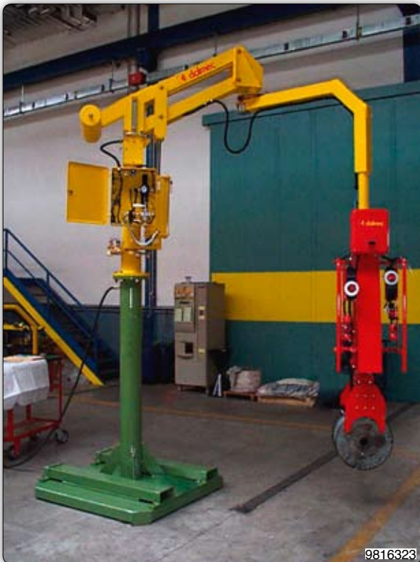
PMC type Partner manipulator, column mounted, provided with pneumatic action gripper for picking coils of wire on flanges with a pneumatic inclination of 90°. Manipulator Partner PMC, 支柱式, 装备气动工具, 可抓取线圈法兰, 可气动旋转90度。
