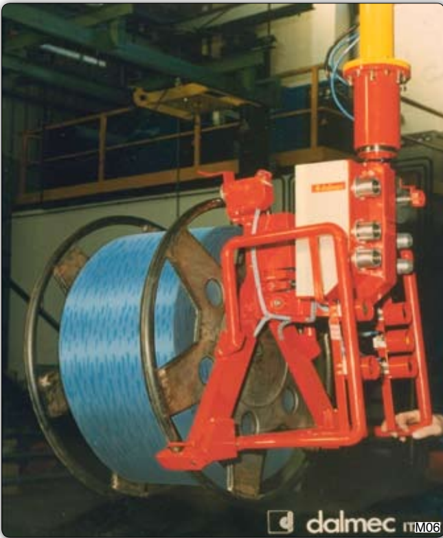
Pneumatic system for picking and moving metal coils. Picking is effected on the flange and the inclination of the coil from the horizontal to the vertical axis is obtained by means of two pneumatic pistons. 气动机械手臂抓取和移动金属线圈。抓取是通过抓住其凸缘来实现，而从水平到垂直倾斜线圈是通过两个气动活塞实现。
