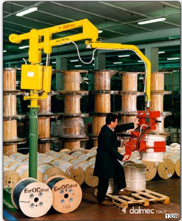
PMC type Partner manipulator, column mounted, equipped with pneumatic action tooling for picking coils of wire on the central belt, with the option of pneumatic inclination from the horizontal to the vertical. Manipulator Partner PMC, 支柱式, 装备气动工具, 可抓取线圈中央带, 另外, 从横向到纵向的气动翻转系统可供选择。
