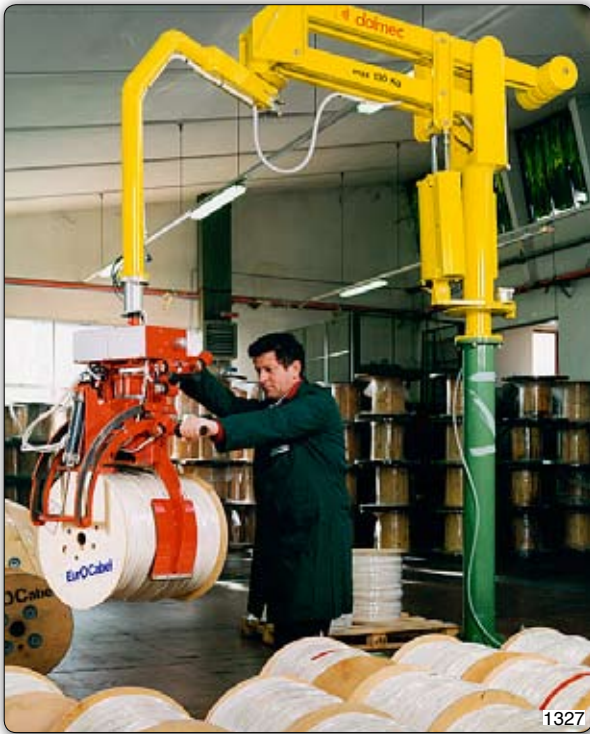
PMC type Partner manipulator, column mounted, equipped with pneumatic action tooling for picking coils of wire on the central belt, with the option of pneumatic inclination from the horizontal to the vertical. Manipulator Partner PMC, 支柱式, 装备气动工具, 可抓取线圈中央带, 另外, 从横向到纵向的气动翻转系统可供选择。
