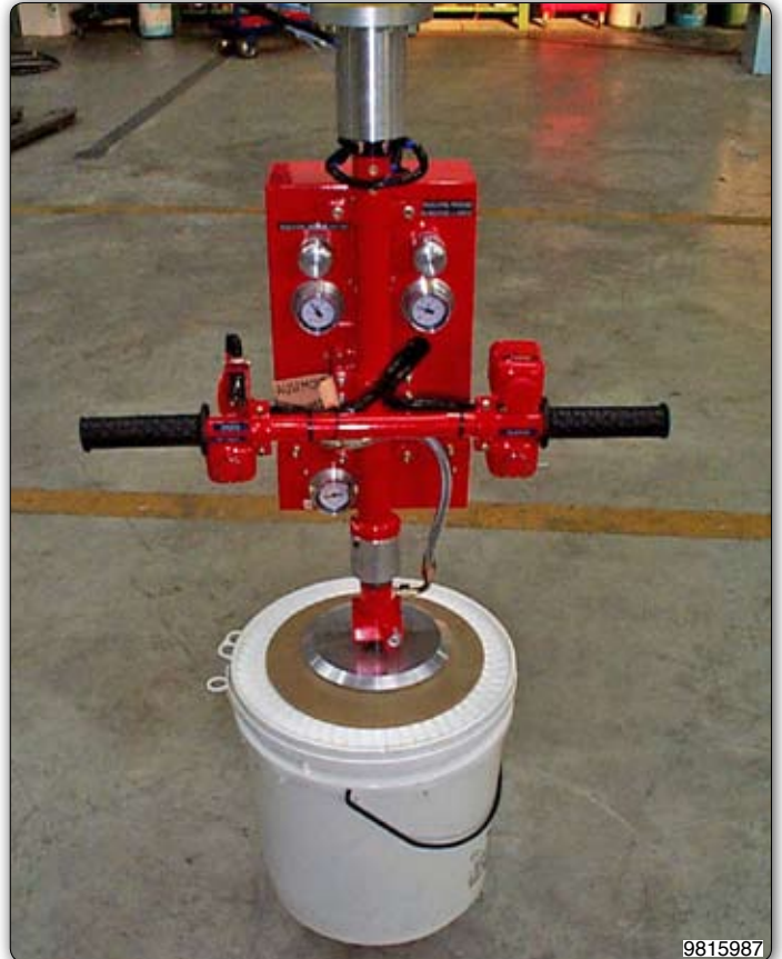
Manipulator equipped with venturi vacuum system for gripping and handling drums. 装备文丘里真空发生器的机械手臂, 用于抓取和搬运圆筒。
