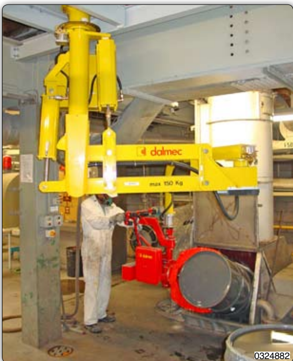
PMF type Partner manipulator, fixed overhead version, designed for the picking and emptying of drums. Manipulator Partner PMF, 墙式, 用于抓取和清空鼓状物体。
