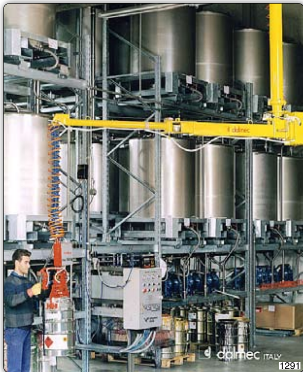
PFF type Posifil manipulator, fixed overhead version for handling metal drums. Manipulator Posifil PFF, 墙式, 用于搬运金属鼓状物体。
