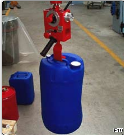
PVC type Posivel manipulator, column design, equipped with specially shaped hook designed for palletizing pails. Manipulator Posivel PVC, 支柱式, 装备特别形状的挂钩, 用于堆积圆筒。
