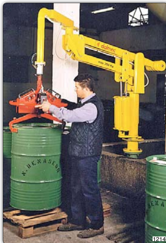
PMC type Partner manipulator, column mounted, equipped with tooling for gripping on the drum's rim. Manipulator Partner PMC 支柱式, 装备可抓取圆筒边缘的工具。
