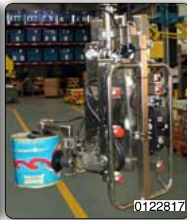
Pneumatic tooling head for handling three drums at the same time. 装备气动工具头，可同时半圆三个圆筒。
