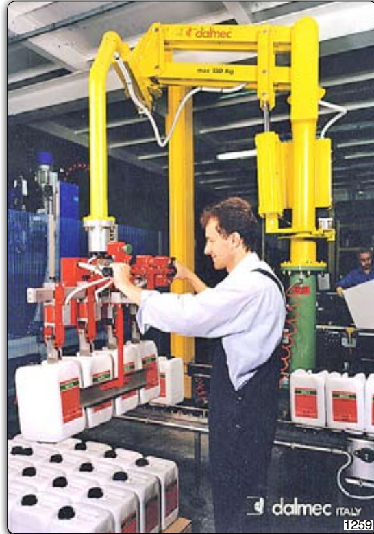
PMC type Partner manipulator, column mounted version, equipped with a pneumatic gripper tooling head to handle four canisters at the same time. Manipulator Partner PMC, 支柱式，气动抓取工具头，可同时搬运四个筒。
