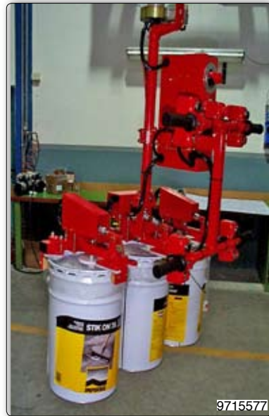
Pneumatic tooling head for handling three drums at the same time. 装备气动工具头，可同时半圆三个圆筒。
