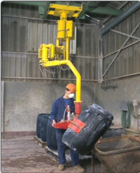
PMS type Partner manipulator, overhead trolley mounted version to cover several work stations, for handling and tipping drums. Manipulator Partner PMS, 高架行车式, 可以覆盖多个工作台, 用于搬运和倾斜圆筒。
