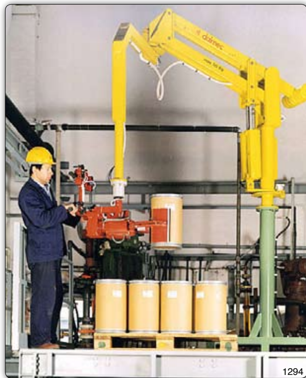
PMC type Partner manipulator, column mounted version, designed for picking and emptying cardboard drums. Manipulator Partner PMC, 支柱式, 专为抓取和清空纸筒而设计。
