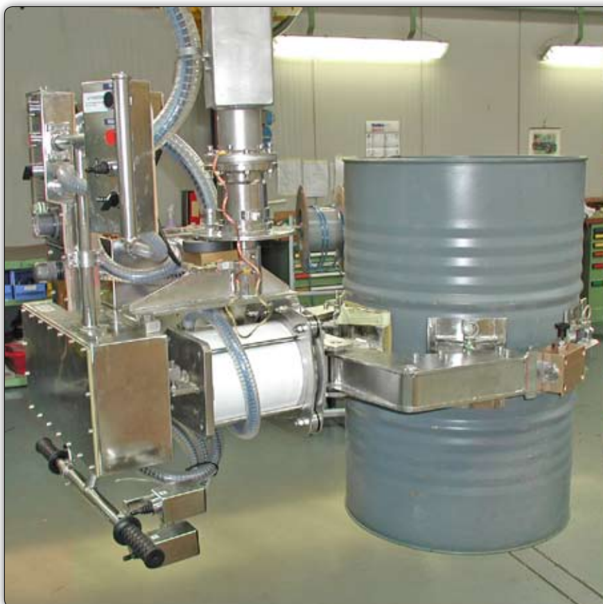
PMC type Partner manipulator, column mounted version, designed for picking and emptying cardboard drums. Manipulator Partner PMC, 支柱式, 专为抓取和清空纸筒而设计。
