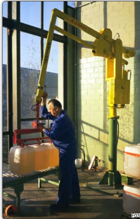
PSC type Partner manipulator, column mounted unit, for handling one or more canisters at once. Manipulator Partner PSC, 支柱式, 用于一次性搬运一个或更多的筒。
