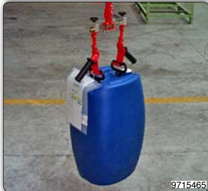
Manipulator equipped with moulded hooks for gripping and handling pails. 装备挂钩的机械手臂, 用于抓取和搬运圆筒。
