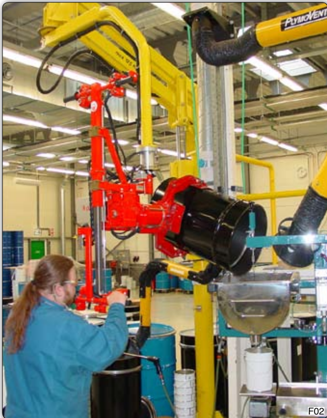
PMC type Partner manipulator, column mounted, designed for the picking and emptying of drums. Manipulator Partner PMC, 支柱式, 用于抓取和清空圆筒。
