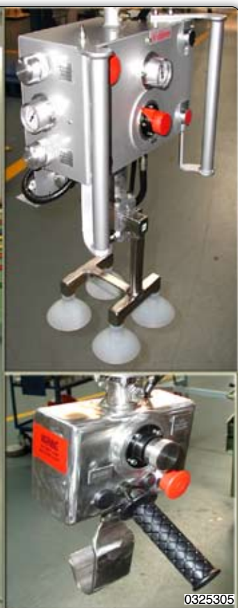
PMC type Partner manipulator, column mounted version, designed for picking and emptying cardboard drums. Manipulator Partner PMC, 支柱式, 专为抓取和清空纸筒而设计。
