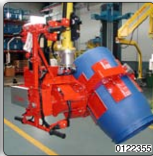
Manipulator with gripper system for picking drums on the rim with dual and low level controls. 装备可抓取圆筒边缘工具机械手臂。
