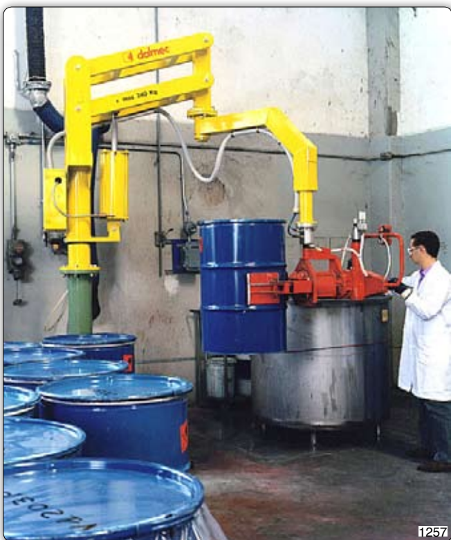
MXC type Maxipartner manipulator, column mounted, made for picking and emptying of drums. Manipulator Partner PMC, 支柱式, 用于抓取和清空圆筒。
