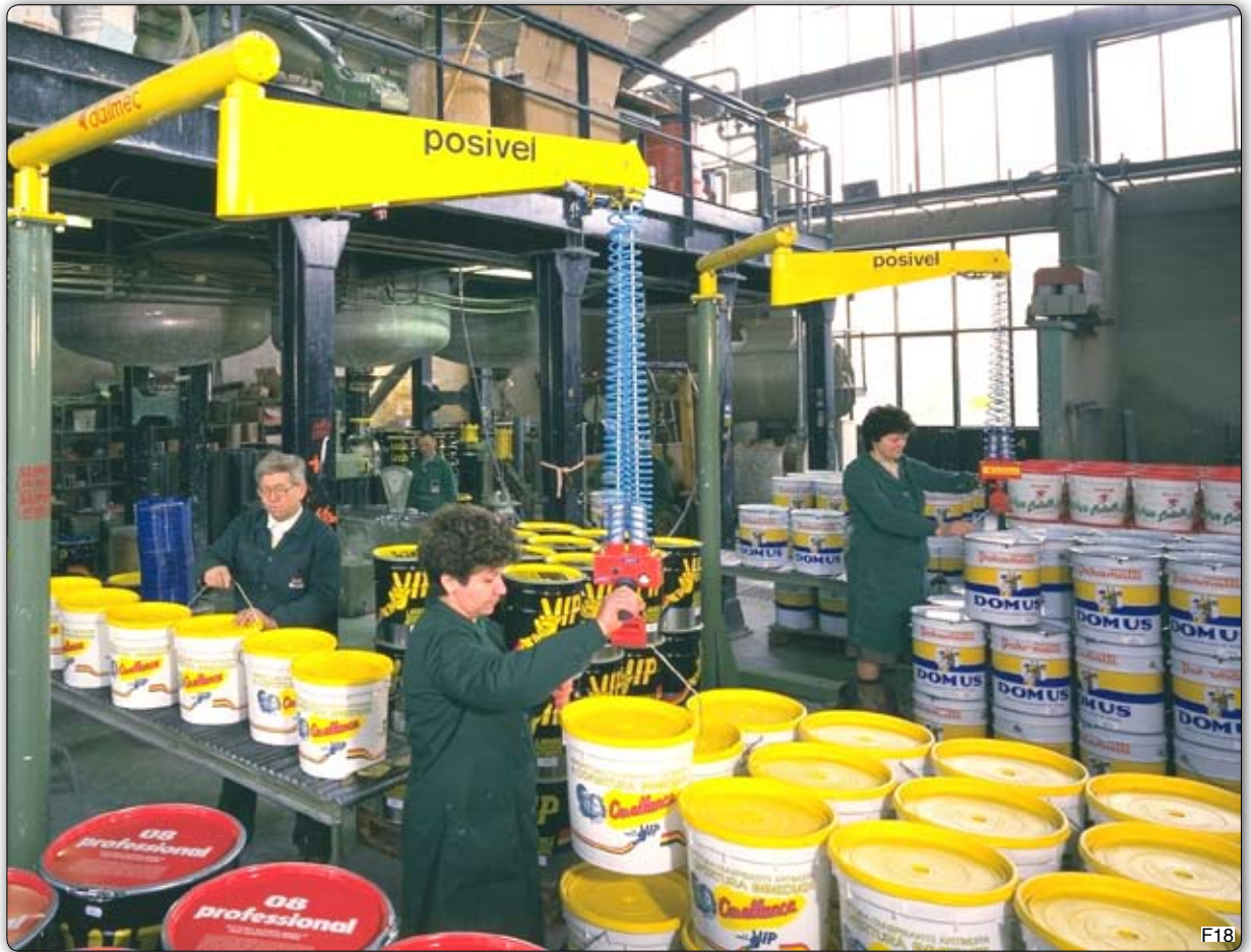
PVC type Posivel manipulator, column design, equipped with specially shaped hook designed for palletizing pails. Manipulator Posivel PVC, 支柱式, 装备特别形状的挂钩, 用于堆积圆筒。
