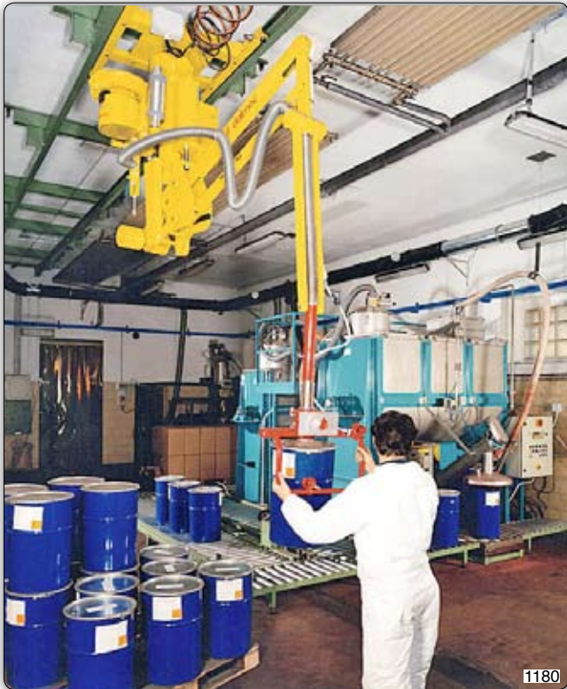
PSS type Partner manipulator, overhead trolley mounted version, with a vacuum tooling head, vacuum being generated by "Venturi" ejector. Partner PSS, 高架行车式，配备真空工具头 真空有文丘里真空发生器产生
