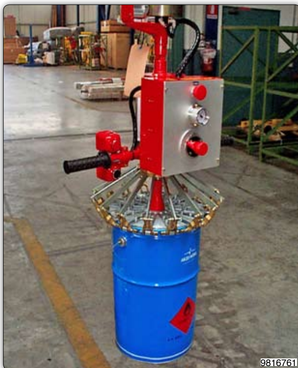
Manipulator equipped with pneumatic tooling for closing and gripping pails on the upper edge. 装备气动工具的机械手臂, 用于封闭和抓取圆筒。
