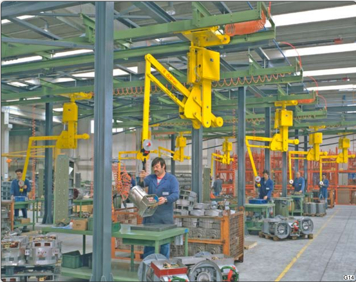
PSS type "Partner" manipulator, overhead trolley mounted machines, used to assemble electric motors. The whole system (tracking system and supporting structure) has been produced by us. Manipulator Partner PSS, 高架行车式, 用于组装电动马达。其轨道和支架结构都有戴尔麦克设计制造。
