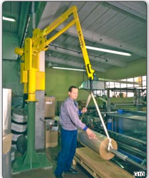
PSC type "Partner" manipulator, column mounted, used to move rolls of plastic film. Manipulator Partner PSC, 支柱式, 用于搬运塑料胶片捆。
