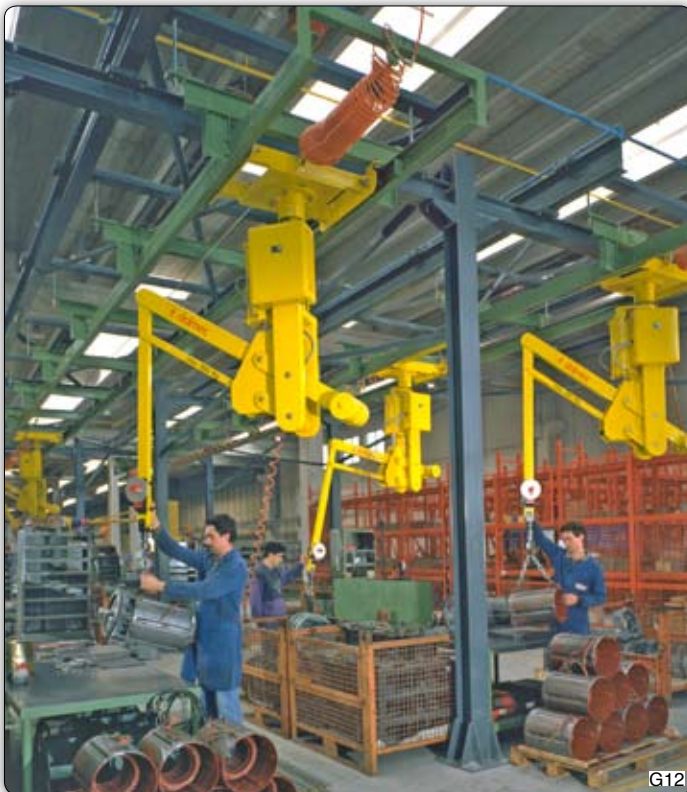
PSS type "Partner" manipulator, overhead trolley mounted, used to assemble electric motors. The tracking system and supporting structure have also been designed and manufactured by Dalmeac. Manipulator Partner PSS, 高架行车式, 用于组装电动马达。其轨道和支架结构都有戴尔麦克设计制造。
