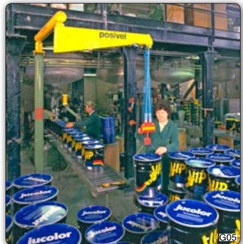
PVC type "Posivel" manipulator, column mounted, equipped with a hook for handling drums. Manipulator tytu Posivel PVC, 支柱式, 装备挂钩, 用于移动筒。
