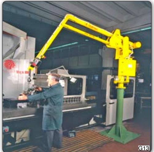
PSC type "Partner" manipulator, column mounted, designed for the loading and unloading of crankshafts from a machining centre. Manipulator Partner PSC, 支柱式, 用于从加工中心搬运曲轴箱。
