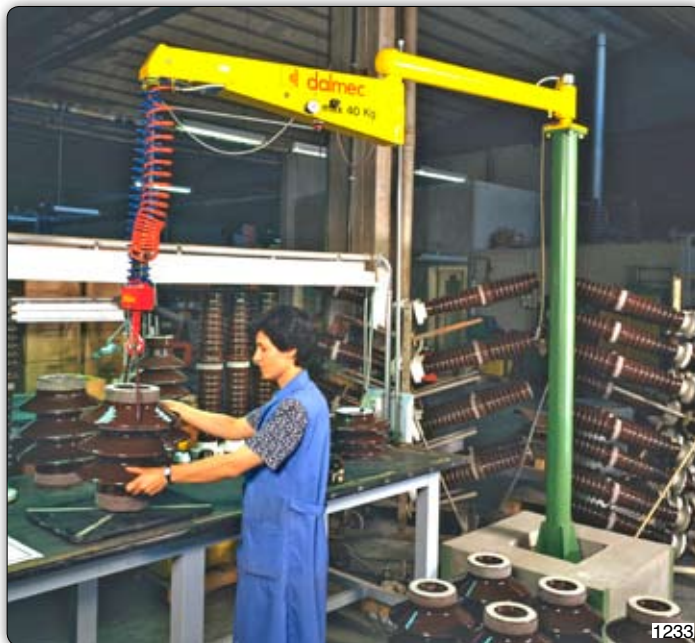
PVC type "Posivel" manipulator, column mounted, used to move isolators. Manipulator tytu Posivel PVC, 支柱式, 用于移动隔离器
