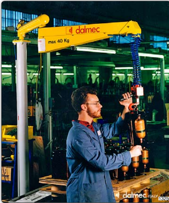
PVC type "Posivel" manipulator, column mounted, used to move refrigeration assemblies for conditioners. Manipulator Posivel PVC, 支柱式, 用于将制冷组建移动到空调上。
