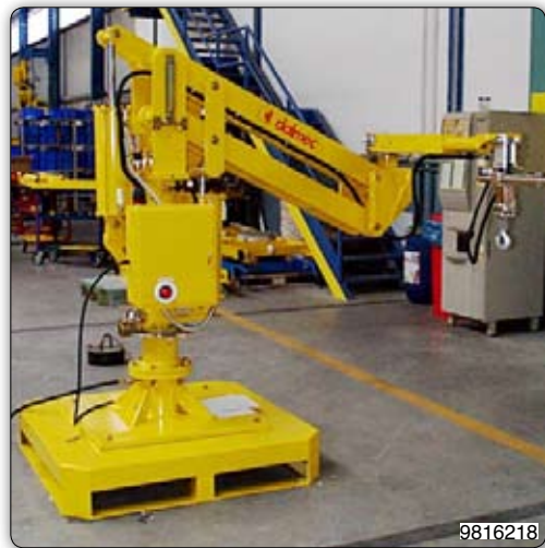
PMC type "Partner" manipulator, low profile version, with stainless steel hook.
