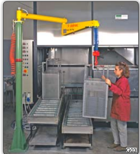
PVC type "Posivel" manipulator, column mounted, designed to move baskets on a washing plant Manipulator Posivel PVC, 支柱式, 用于将滚筒移动到洗衣机上
