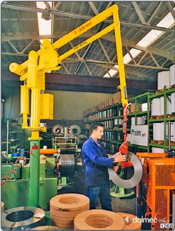
PSC type "Partner" manipulator, column mounted used to move rolls of band strapping. Manipulator Partner PSC, 支柱式, 用于移动卷带捆包
