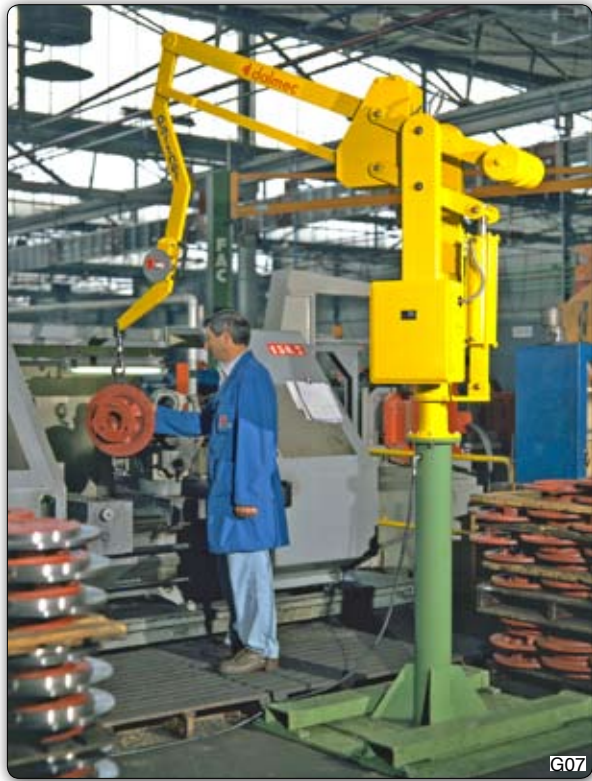
PSC type "Partner" manipulator, column mounted with gooseneck terminal arm, used to move epicycloidal spiders. Manipulator tytu Partner PSC, 带有鹅颈臂支柱式, 用于搬运网状物
