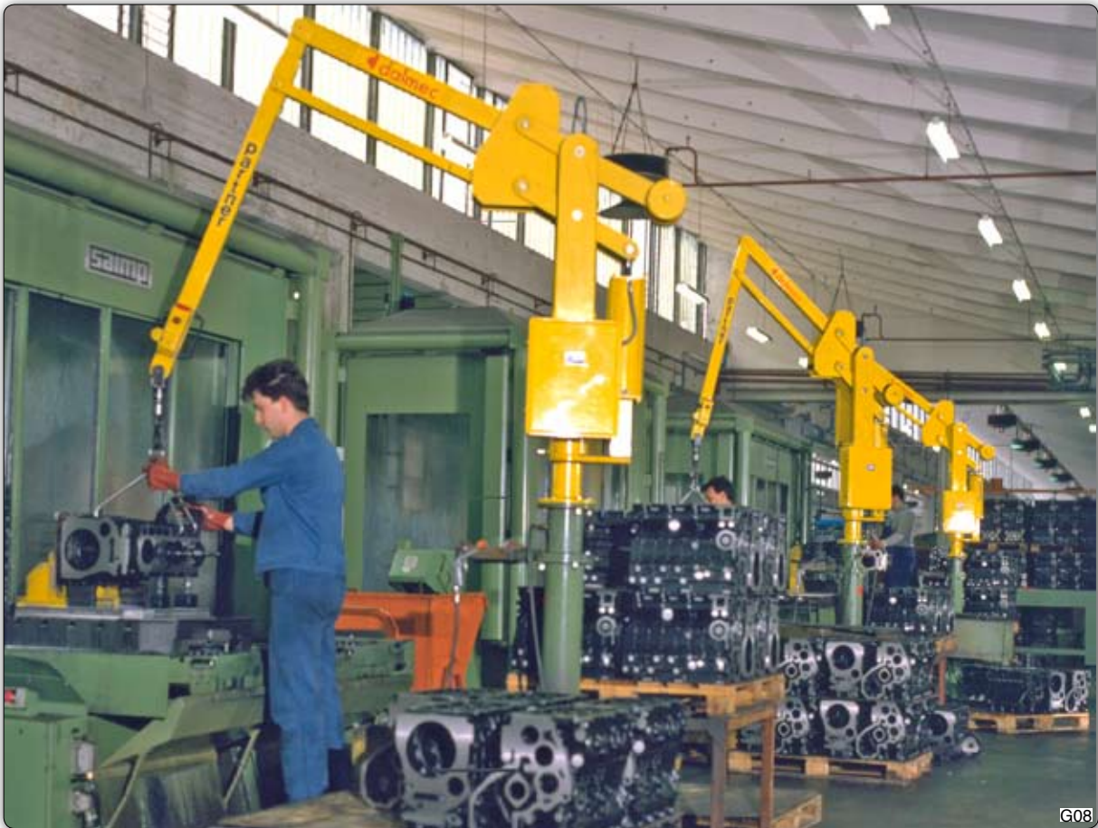
PSC type "Partner" manipulators, column mounted, used to move crankcases between various workstations. Manipulator Partner PSC, 支柱式, 用于在工作台间搬运曲轴箱。
