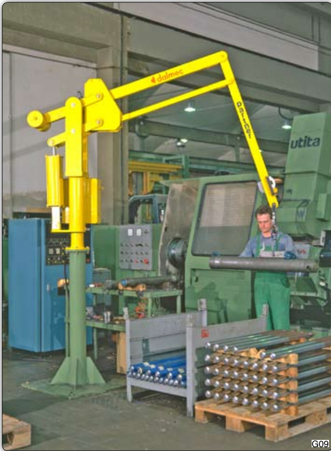
PSC type "Partner" manipulator, column mounted with extended parallelogram, used to move oleodynamic cylinders over a workstation. Manipulator Partner PSC, 支柱式用于在工作台上搬运气瓶。
