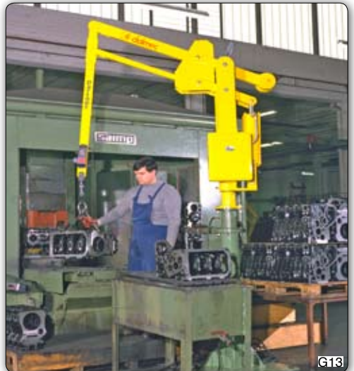
PSC type "Partner" column mounted, used for handling crankcases onto a de-greasing plant. Manipulator Partner PSC, 支柱式, 用于将曲轴箱搬运到润滑工厂。
