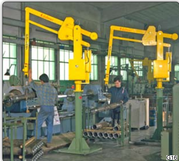
PSC type "Partner" manipulators, column mounted, used to position hydraulic cylinder barrels onto machine tools. Manipulatory Partner PSC, 支柱式, 用于将气罐放入机器中。
