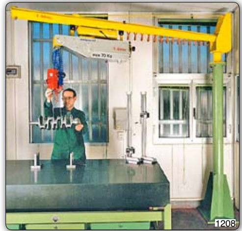
MPC type "Minipartner" manipulator, flag-type column mounted unit, used to move crankshafts to a measuring bench. Manipulator Minipartner MPC, 支柱式, 用于将机轴移动到测量台上。
