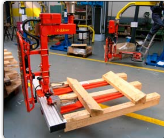
Adjustable forks tooling with pneumatic rotation of the load and telescopic controls. 可调节的叉形工具，可气动翻转栈板，并可远控。
