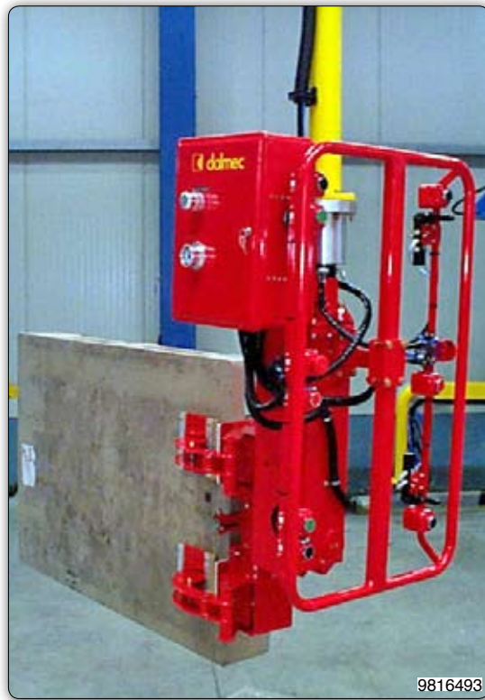
Manipulator with jaws tooling for pneumatic rotation of the pallet. 装备卡爪机械手臂，可以气动旋转栈板。
