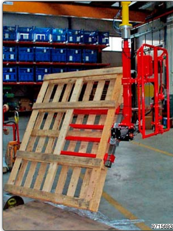
Manipulator with forks type tooling with 180° pneumatic rotation for gripping and overturning pallets.
