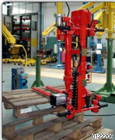
Adjustable forks tooling with pneumatic rotation of the load and telescopic controls. 可调节的叉形工具，可气动翻转栈板，并可远控。
