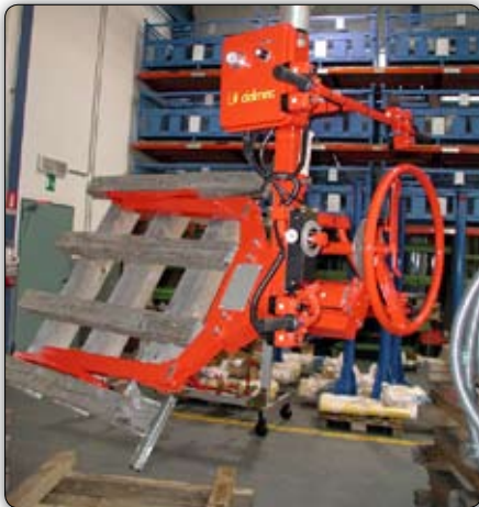
Manipulator with particular forks for gripping and handling stainless steel pallets. 特制叉手的机械手臂，抓取和搬运不锈钢栈板。
