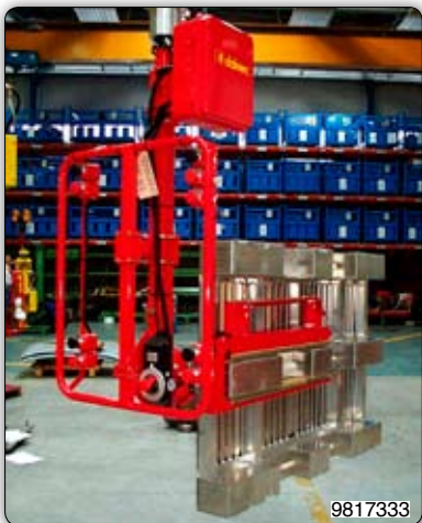
Manipulator with particular forks for gripping and handling stainless steel pallets. 特制叉手的机械手臂，抓取和搬运不锈钢栈板。
