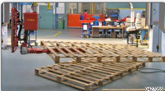
Manipulator with jaws type tooling and manual rotation of particular pallets. 装备卡爪机械手臂，可以手动旋转特殊栈板。
