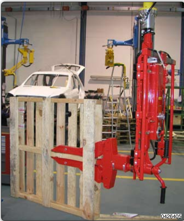
Manipulator with pneumatic tooling with manual of the pallet. 装备气动工具的机械手臂，可以抓取栈板。
