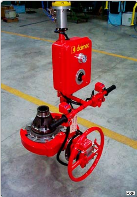
Manipulator with equipment for moving wheel hubs with 180° manual rotation. Manipulator 用于搬运轮毂并180度手动旋转。
