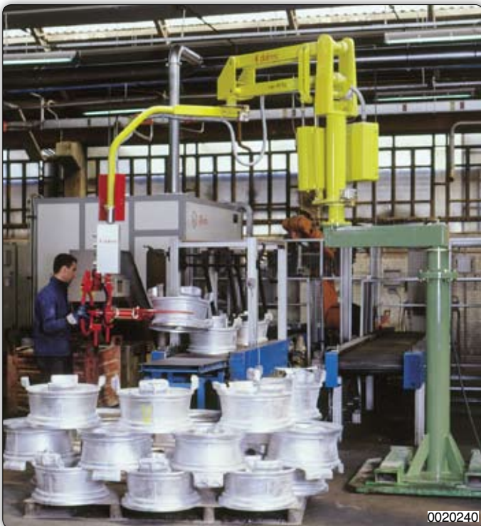
PMC type Partner, column mounted manipulator, with gripper equipment, made for taking and moving tractor rims of various sizes. Manipulator Partner PMC, 支柱式, 装备抓手, 用于搬运各种尺寸的拖拉机轮胎
