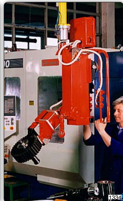
PMC type Partner manipulator, column design, with special equipment for picking, inclination and rotation of gears. Manipulator Partner PMC, 支柱式, 配备特殊设备以便抓取, 倾斜和旋转齿轮。
