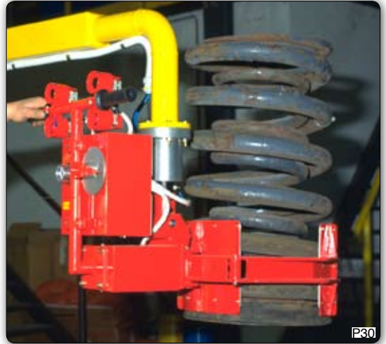
Manipulator with gripper equipment for picking the complete suspension of a railway carriage and the relative positioning in a dynamic testing machine. Manipulator
