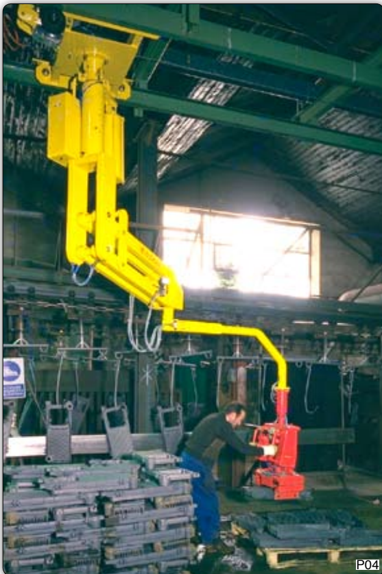
PMS type Partner manipulator, overhead trolley mounted, complete with pneumatic gripper tooling for the movement of boiler components, suitable for picking and moving components from an overhead conveyor, and following 90° pneumatic inclination, for placing these on a pallet. The overhead tracking is also made by Dalmecc.
