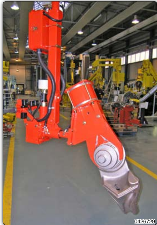
Pinch jaws tooling for the gripping and pneumatic rotation of milling machines parts having different forms and weights. 卡爪，用于抓取和气动旋转不同尺寸和重量的铣床元件。
