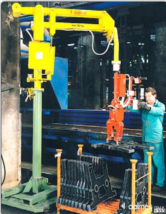
PMC type Partner manipulator, column design with special gripper equipment for taking smelted items from a conveyor belt. Manipulator Partner PMC, 支柱式, 配备特殊抓手, 用于从传送带上搬运高温物品。
