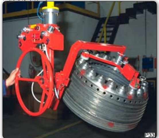
Manipulator with equipment for loading and unloading of aero engine collectors from a welding plant. A steering wheel on a equipment enables manual inclination of the collectors. Manipulator 用与在焊接厂装卸航空发动机集电器。在此机械手臂上装手轮子以便手动倾斜集电器。
