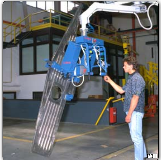
Manipulator with gripper equipment and pneumatic systems for 90° inclination and 180° rotation, for moving specific items from aircraft wings. Manipulator 装备抓手和可以将物体90度倾斜和180度线转的气动系统, 用于从飞机上搬运特殊物品。
