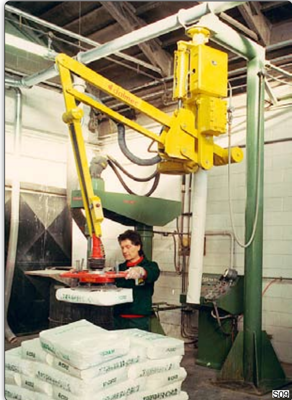
PSC type Partner manipulator, fixed version, used to move bags from a sack filler to a pallet. Manipulator Partner PSC, 墙式, 用作将包装机的产品搬运到栈板上。
