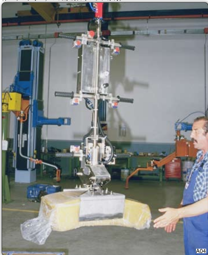
Manipulator with pneumatic jaws for handling rubber bales. The "slimline" design of the jaws allows for easy release into the bale's packaging. 装备气动卡爪的机械手, 用于搬运橡胶包。 “苗条”的卡爪可以很轻易的抓紧橡胶包。
