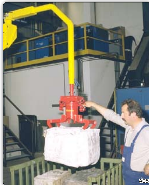
Manipulator with pneumatically actuated grippers, which hold the bale by gripping into the product itself. 装备气动卡爪抓取包状物体的机械手
