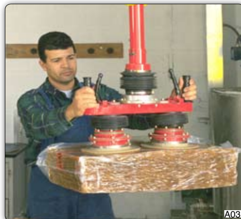
Tooling head for handling rubber bales with independently swivelling suction cups. 使用独立的转动吸盘搬运多个橡胶包的工具头。
