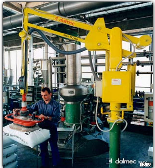
PSC type Partner manipulator, column mounted, equipped with suction head to pick bags from a pallet and loading them to a mixer. Manipulator Partner PSC, 支柱式, 装备吸盘, 可从栈板上吸附包状物体, 并将其放进混合器里。
