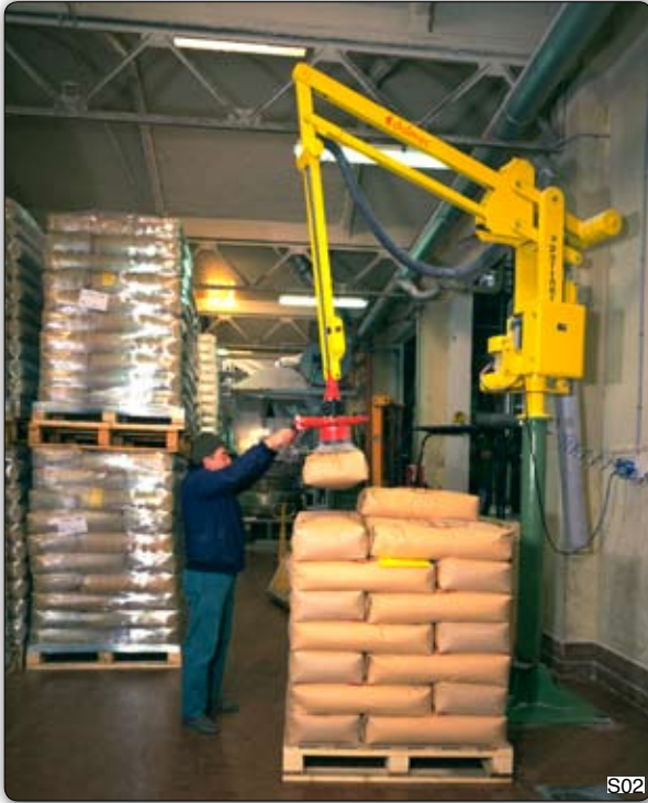
PSC type Partner manipulator, column mounted for palletization/depalletization of bags which are stacked up to about metres from floor level, fitted with lowered controls. Manipulator Partner PSC, 支柱式, 装备降低控制装置, 用于将包状物体装卸到栈板上, 并可将其堆积数米高。
