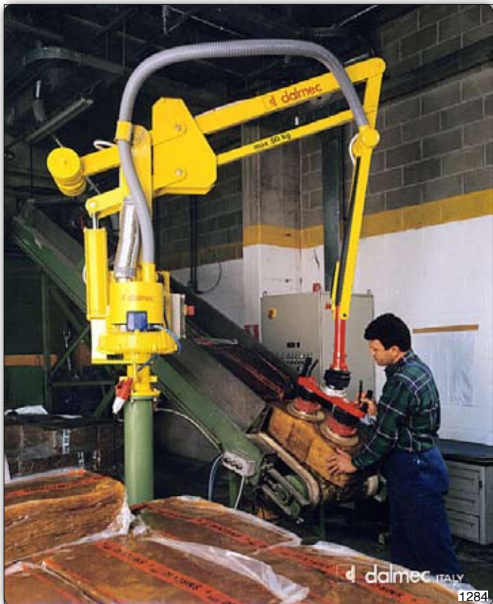
PSC type Partner manipulator, column mounted, with suction head for handling rubber bales used for a trituration plant, equipped with an "extra pull" feature to facilitate detachment of the bale from the one underneath it. Manipulator Partner PSC, 支柱式, 装备吸盘, 搬运用于研磨设备所需要的橡胶包, 装备另一个“拉手”, 以便橡胶捆可以轻松分离。
