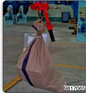
PSC type Partner manipulator, column mounted, equipped with suction head to pick bags from a pallet and to load them to a mixer. Manipulator Partner PSC, 支柱式, 装备吸盘, 从栈板上吸附包状物体, 并将其放进混合器里。
