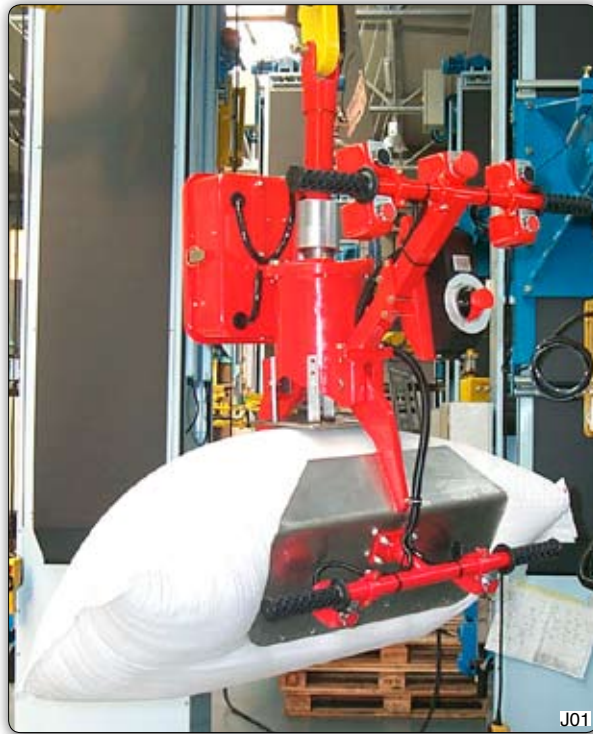
Manipulator with pneumatically actuated gripper picking system. 装备气动卡爪的机械手
