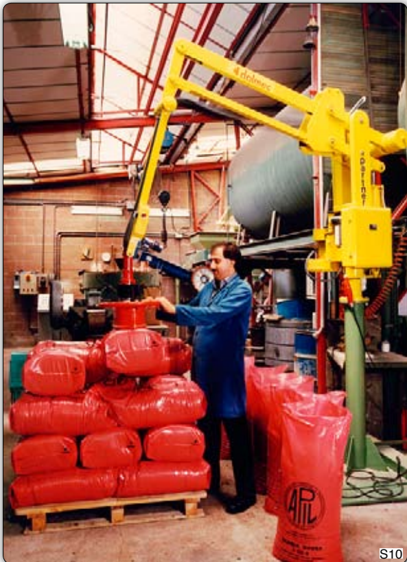
PSC type Partner manipulator, column design, overhead used to move bags from a sack filler to a pallet. Manipulator Partner PSC, 支柱式, 用作将袋灌装机的产品搬运到货架上。
