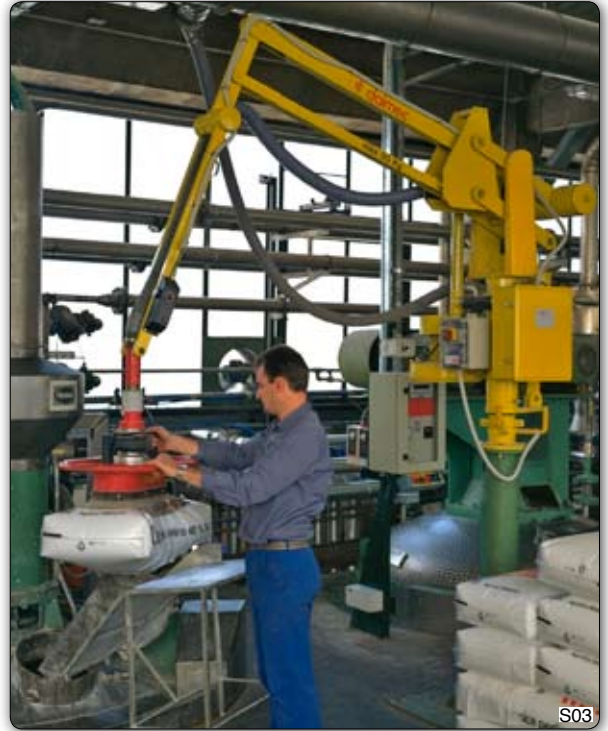
PSC type Partner manipulator, column mounted, equipped with suction head to pick bags from a pallet and to load them to a mixer. Manipulator Partner PSC, 支柱式, 装备吸盘, 从栈板上吸附包状物体, 并将其放进混合器里。
