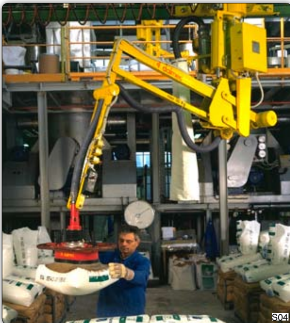
PSS type Partner manipulator, overhead trolley mounted version in Dalmec track. The operator picks bags from various pallets in the "picking" area and deposits them to a common pallet. Manipulator Partner PSS, 高架行车式, 配备戴尔麦克制造的轨道, 操作人员从抓取区各种栈板上抓取包状物体, 并将它们放在
