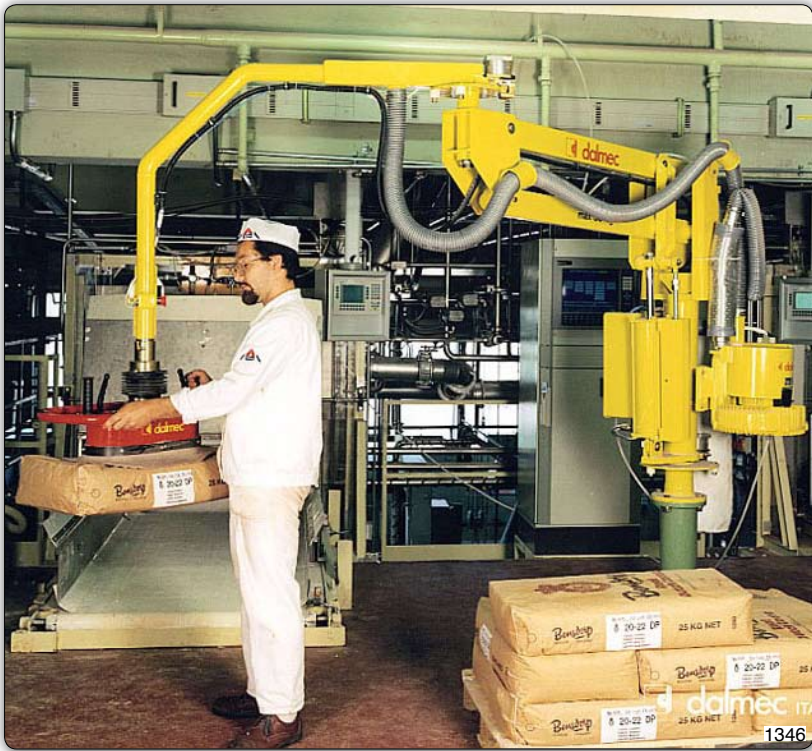
PMC type Partner manipulator, column design, special low profile unit, to enable to operate in a room with low ceiling. The equipment allows the bags to be picked from a pallet and to be loaded onto a hopper. Manipulator Partner PMC, 支柱式, 特殊紧凑型, 在低房顶的空间中使用。此设备从栈板上抓取包状物体并将其放在送料斗中。
