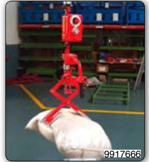
PSC type Partner manipulator, column mounted, equipped with suction head to pick bags from a pallet and to load them to a mixer. Manipulator Partner PSC, 支柱式, 装备吸盘, 从栈板上吸附包状物体, 并将其放进混合器里。
