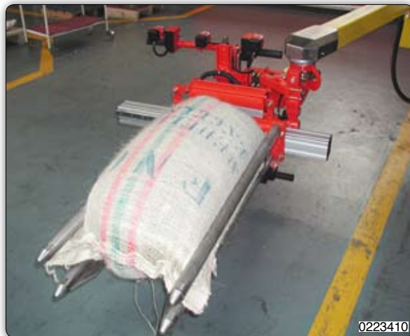
Manipulator with pneumatically actuated gripper picking system. 装备气动卡爪的机械手
