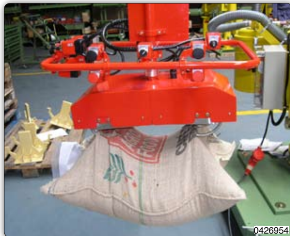
Manipulator with retractable hooks for handling hessian sacks. 装备可收缩吊钩的机械手，用于搬运大包货物。
