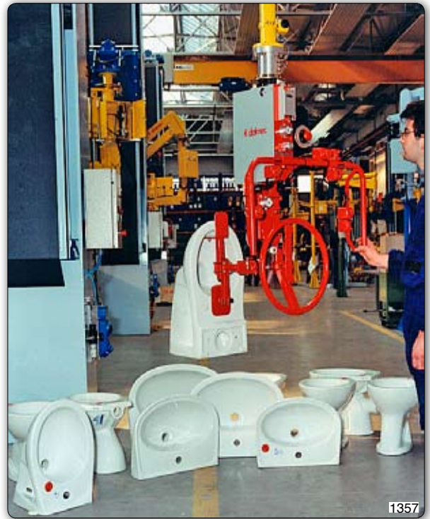
Manipulator with suction cup tooling for gripping and manual rotation of WC. Manipulator 配备气动工具, 用于抓取和旋转卫浴用品。
