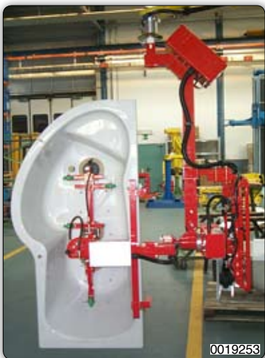
Suction cups (Venturi) Manipulator for gripping and rotation of bathtubs. Manipulator 装备文丘里吸盘，用于抓取和旋转浴缸。
