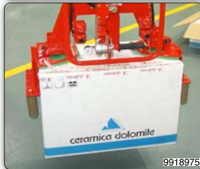
Manipulator with jaws tooling for gripping sanitary, their releasing into the cartons, gripping the packaged boxes and their pallettization. Manipulator 装备钳口, 可将包装过的卫浴用品搬运和装卸到卡车里。
