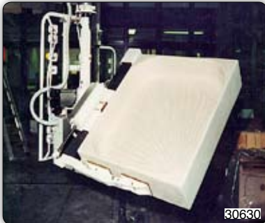
Manipulator with pneumatic tooling for gripping and rotation of shower plates. Manipulator 装备气动工具, 用于抓取和旋转淋浴板。
