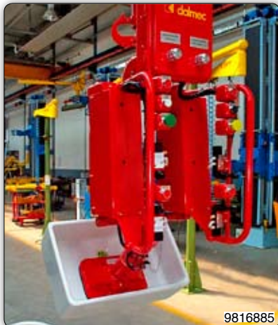
Manipulator with suction cups tooling (Venturi) for gripping and inclination of sinks. Manipulator 装备文丘里吸盘，用于抓取和倾斜洗脸槽。
