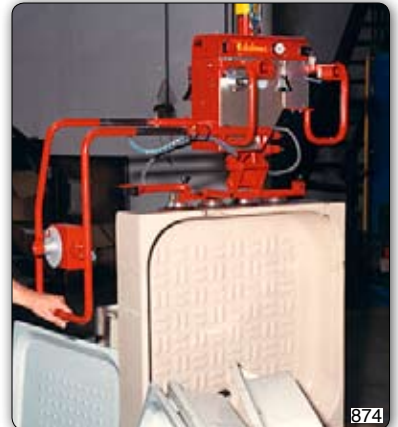
PMF Partner Manipulator, fixed overhead, with suction cups tooling (Venturi) for gripping and manual rotation of shower plates. Manipulator Partner PMF, 悬壁式, 装备文丘里吸盘, 用于抓取和倾斜淋浴板。
