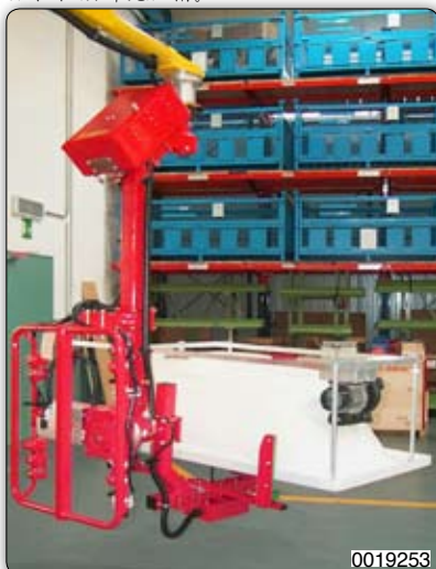
Suction cups (Venturi) Manipulator for gripping and rotation of bathtubs. Manipulator 装备文丘里吸盘，用于抓取和旋转浴缸。
