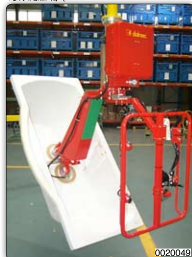
Suction cups Manipulator (Venturi) for gripping and inclination of bathtubs. Manipulator 装备文丘里吸盘，用于抓取和倾斜浴缸。
