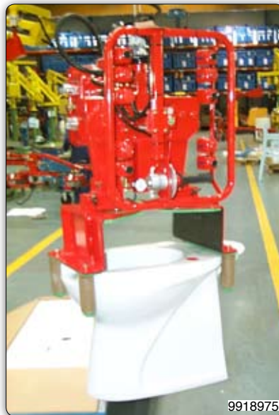
PMF Partner Manipulator, fixed overhead, with interchangeable suction cups tooling for gripping and handling sinks having different dimensions. Manipulator Partner PMF, 墙式, 配备可更换的吸盘, 用于抓取和搬运不同尺寸的水槽。
