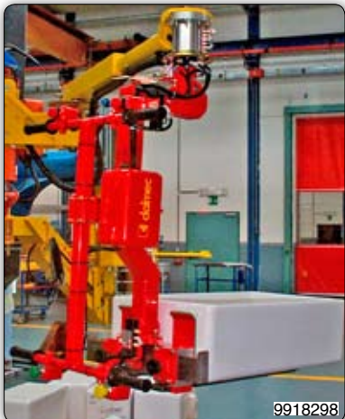
Manipulator with forks type tooling for handling sinks. Manipulator 装备叉，可搬运洗脸槽。
