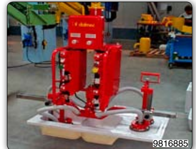
Manipulator with adjustable suction cups tooling (Venturi) for handling and inclination of sinks. Manipulator 装备文丘里吸盘, 用于抓取和倾斜洗脸槽。
