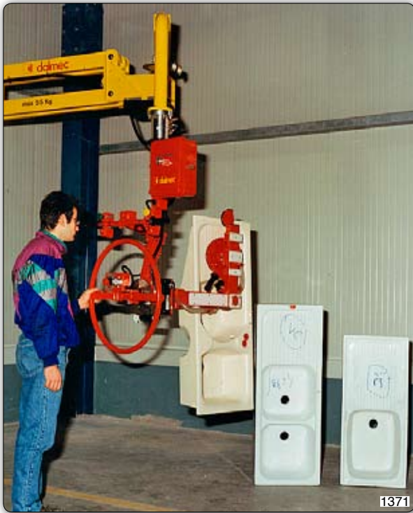
PMF Partner Manipulator, fixed overhead, with interchangeable suction cups tooling for gripping and handling sinks having different dimensions. Manipulator Partner PMF, 墙式, 配备可更换的吸盘, 用于抓取和搬运不同尺寸的水槽。
