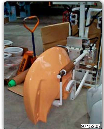
Manipulator with adjustable forks type tooling for gripping and handling sinks. Manipulator 备有可调节叉, 用于抓取和搬运洗脸槽。
