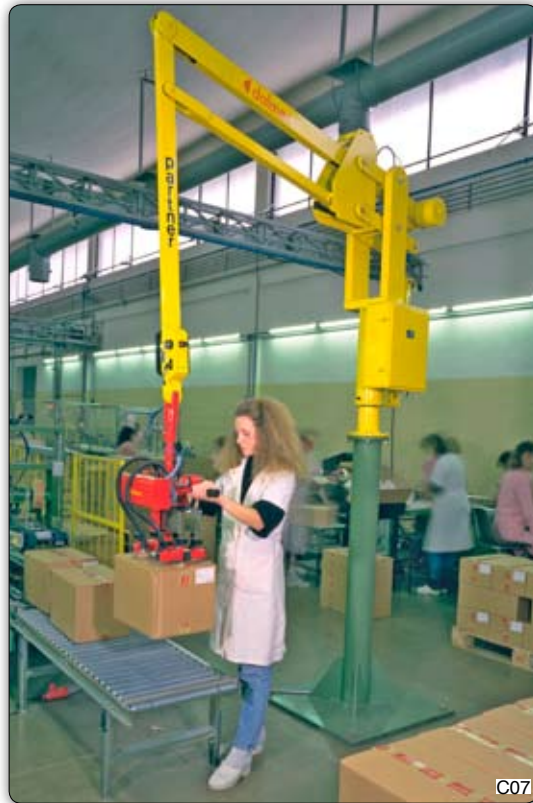
PSC type Partner manipulator, column mounted, equipped with a Venturi vacuum suction system. Manipulator Partner PSC, 支柱式, 装备文丘里真空吸盘装置。
