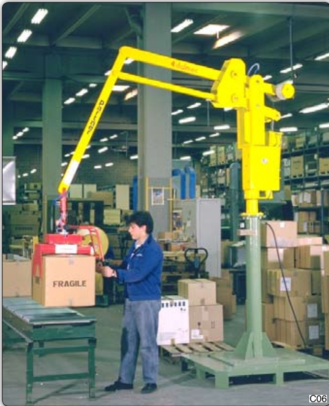
PSC type Partner manipulator, column mounted, equipped with jaws gripping system, for the picking and palletization of boxes packed with household electric appliances of various types and weights. Manipulator partner PSC, 支柱式, 装备钳口抓取系统, 可抓取和装卸各种类型和重量的家用电器包装箱。
