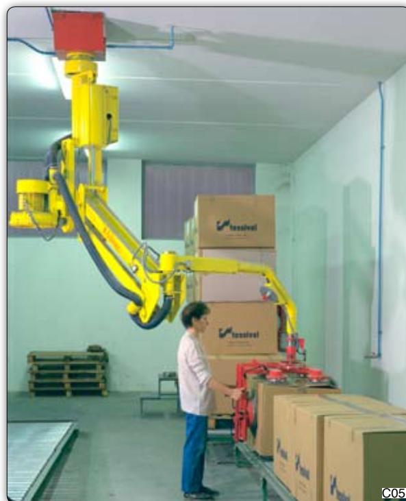
PMF type Partner manipulator, fixed overhead, equipped with suction system to grip and handle cardboard boxes from the packaging lines to pallets.
