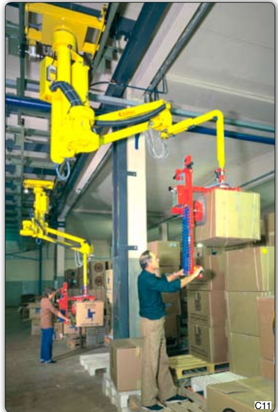
PMS type Partner manipulator, overhead trolley mounted, with motorised pneumatic drive, equipped with special suction head and telescopic commands to allow the operator to pick boxes from a high stack on a pallet. Manipulator Partner PMS, 高架行车式, 气动马达, 装备特殊吸盘和伸缩装置, 可以从货架高处提取货物。
