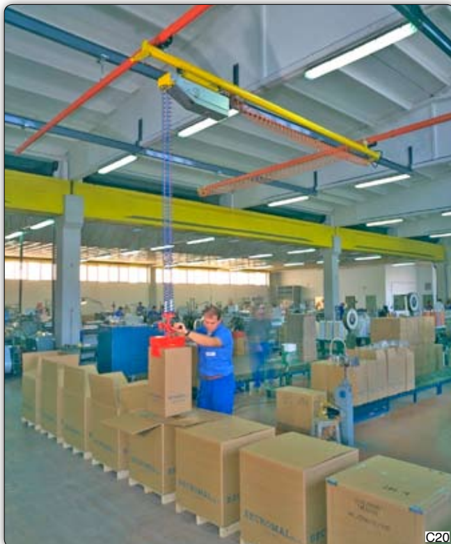
MPS type Minipartner manipulator, overhead trolley mounted, equipped with pneumatic jaws for gripping and handling boxes of different dimensions and weights. The tooling is fitted with a proportional valve to allow the operator to easily set the balancing system. The overhead trolley and downshop tracking system are made by Dalmec. Manipulator Minipartner MPS, 高架行车式, 装备气动钳口, 可抓取和搬运不同尺寸和重量的箱包。此设备上装备平衡阀使操作人员轻松平衡系统。高架轨道有戴尔麦克制造。
