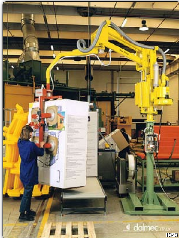
PMC type Partner manipulator, column mounted, fitted with suction tooling to grip and handle cardboard boxes from a packaging line to a pallet. Manipulator Partner PMC, 支柱式, 装备吸附工具, 从传送带上搬运箱包到货架上。
