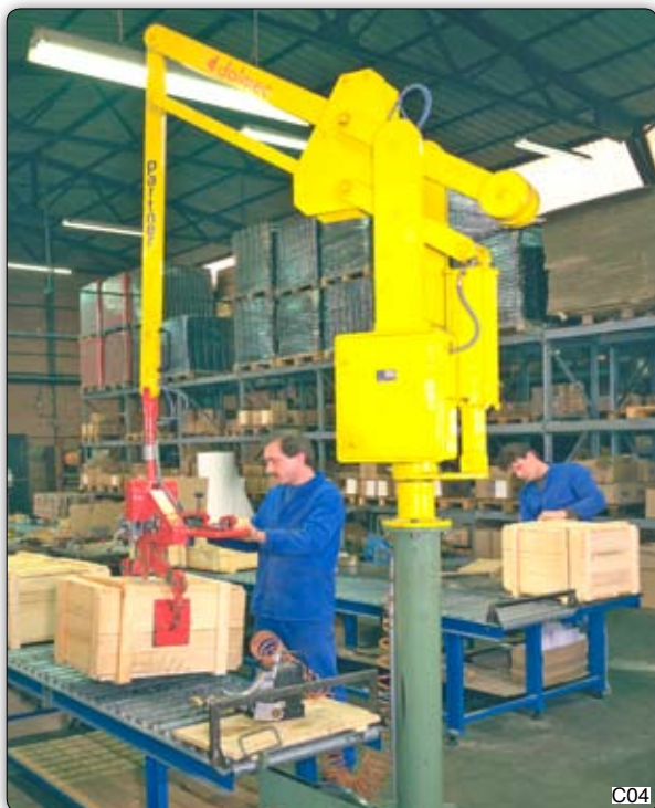
PSC type Partner manipulator, column mounted, fitted with pneumatic gripper tooling. The special design of the tooling jaws allows the handling of a particularly wide range of wooden cases.
