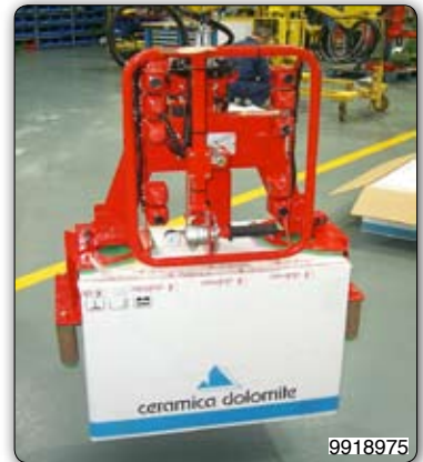
PFC type "Posifil" manipulator, column design, equipped with gripper system for picking sanitary ware, inserting it in cardboard boxes, picking the packed boxes and putting them on to pallets. Manipulator Posifil PFC, 支柱式, 装备抓取系统, 用于抓取卫生洁具, 并将其塞入木箱中, 并可以将包装好的木箱搬运到货架上。
