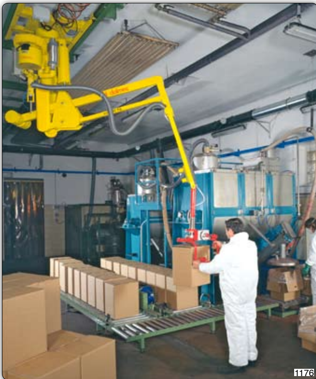
PSS type Partner manipulator, overhead trolley mounted version, fitted with vacuum tooling for gripping boxes from one packaging line and positioning the same on a pallet. The overhead tracking system is manufactured by Dalmecc. Manipulator Partner PSS, 高架行车式, 装备真空吸盘, 可以从装配线抓取箱包并将其放在货架上。高架轨道有戴尔麦克制造。
