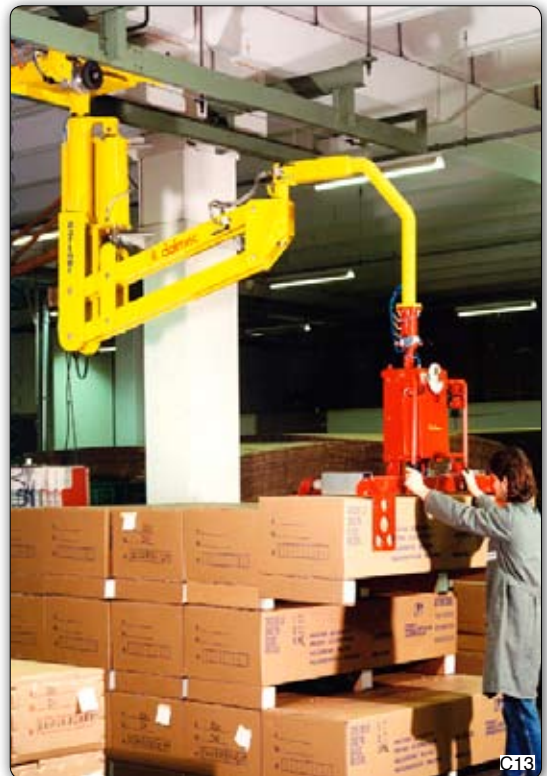
PMS type Partner manipulator, overhead trolley mounted, with motorised pneumatic drive, equipped with special gripper tooling, which allows the operator for gripping and 90° inclination of the box, so that pins can be fitted under the same. It is also completed with tracking system made by Dalmecc.
