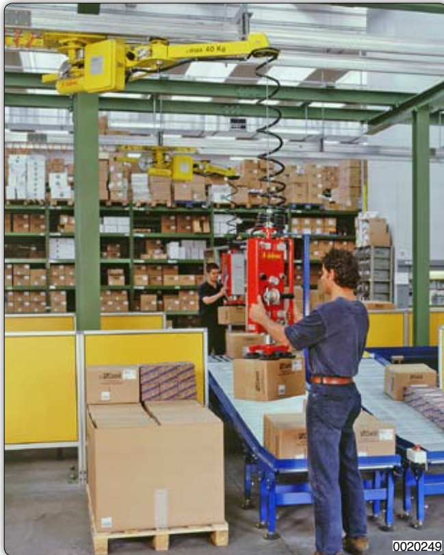
SPS type Speedyfil manipulator, overhead trolley mounted, equipped with a Venturi vacuum suction system. Manipulator Speedyfil SPS 高架行车式, 装备文丘里真空吸附设备。
