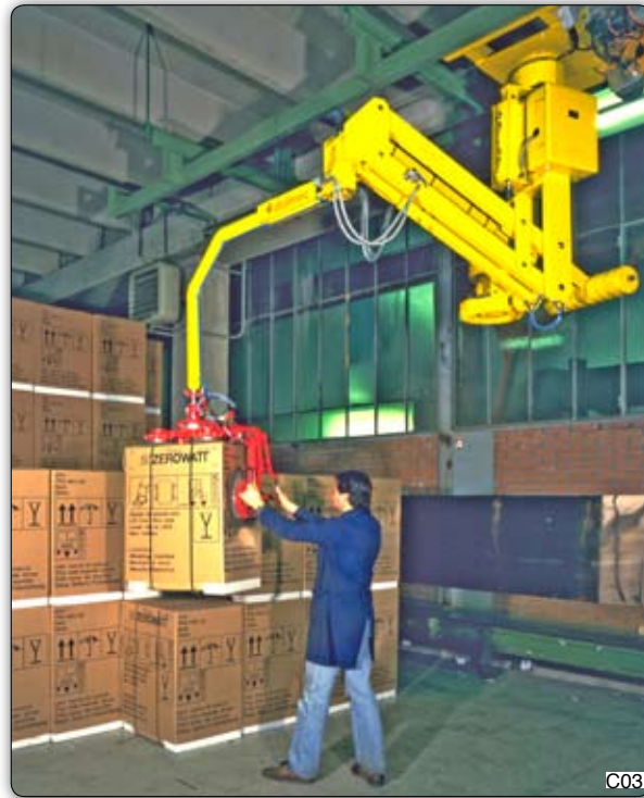
PMS type Partner manipulator, overhead trolley mounted, suitable for stacking boxes containing a variety of washing machines which arrive from the packaging line. A pneumatic motor drive is also fitted to the system, which runs in Dalmec overhead tracking.
