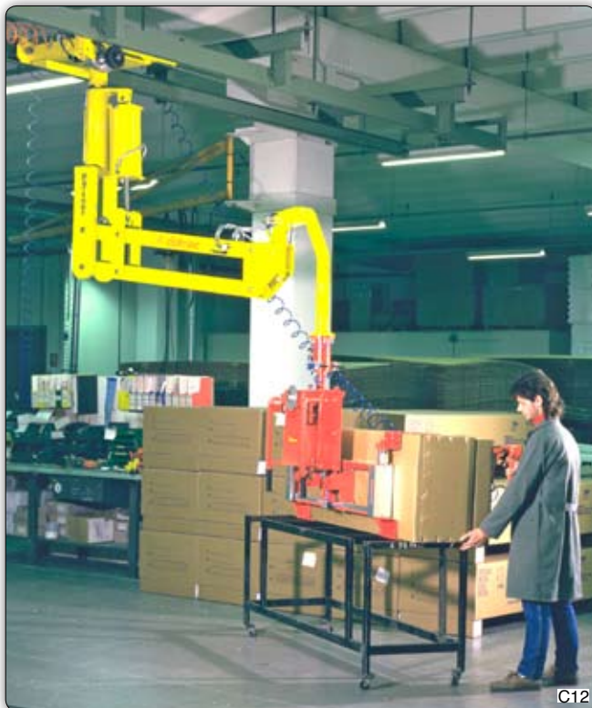
PMS type Partner manipulator, overhead trolley mounted, with motorised pneumatic drive, equipped with special gripper tooling, which allows the operator for gripping and 90° inclination of the box, so that pins can be fitted under the same. It is also completed with tracking system made by Dalmecc.
