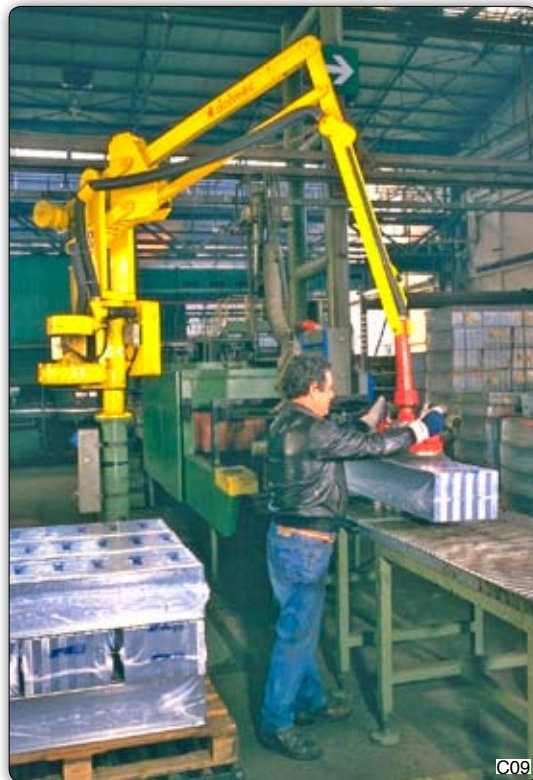
PSC type Partner manipulator, column mounted, fitted with suction cups tooling for gripping shrink-wrapped goods from a packaging line to a pallet. Manipulator Partner PSC, 支柱式, 装备真空吸盘, 可以从装配线抓取箱包并将其放在货架上。
