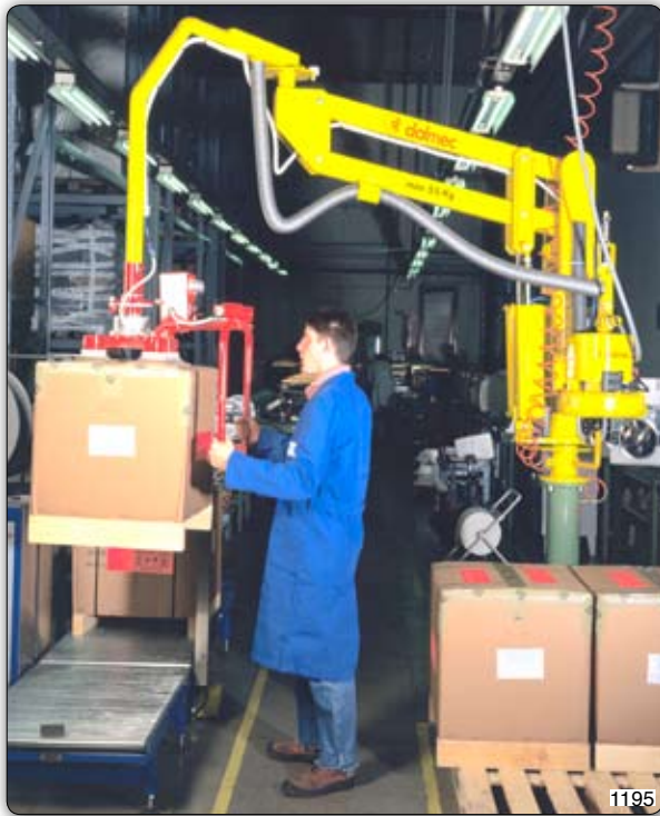
PMC type Partner manipulator, low profile model, fitted with suction head for gripping cardboard boxes and designed to operate in an area with a low ceiling. Manipulator partner PMC, 紧凑型, 装备吸盘, 用于抓取箱形物体, 专为低矮厂房设计。
