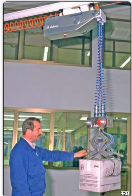
MPS type Minipartner manipulator, with overhead balancer unit, handling blocks of butter, both with and without packaging. The tooling is made of stainless steel, and the pneumatic grippers are controlled by a pressure regulator. Manipulator Minipartner 装备间接平衡器, 搬运包装或未包装的黄油。此设备由不锈钢制成, 气动抓手又压力调节器控制。
