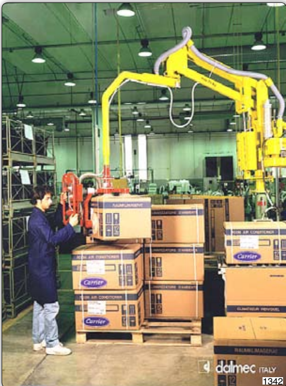
PMC type Partner manipulator, column mounted, with suction gripping system, a popular design, commonly used for moving packing boxes from a conveyor belt to a pallet. Manipulator Partner PMC, 支柱式, 装备吸盘, 一般用于从传送带抓取货物到货架上。
