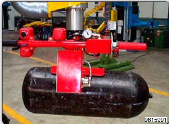
Manipulator with suction cup tooling (Venturi) for gripping and releasing the tanks into the car. 装备真空吸盘（文丘里）的机械手，用于将气瓶搬运安装在汽车上。
