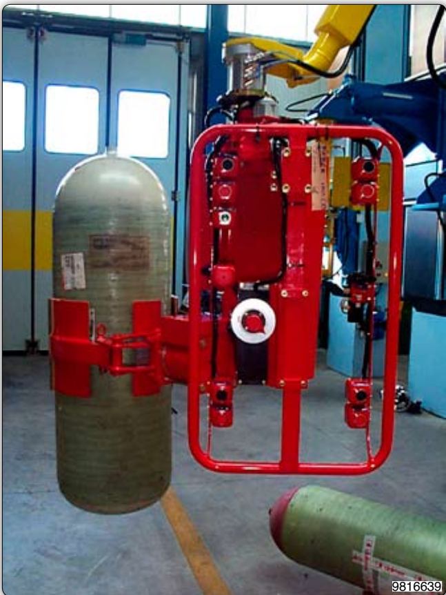
Manipulator with pneumatic tooling for gripping and inclination of cylinders having different dimensions. 装备气动工具的机械手臂，用于抓取和倾斜不同尺寸的气缸。
