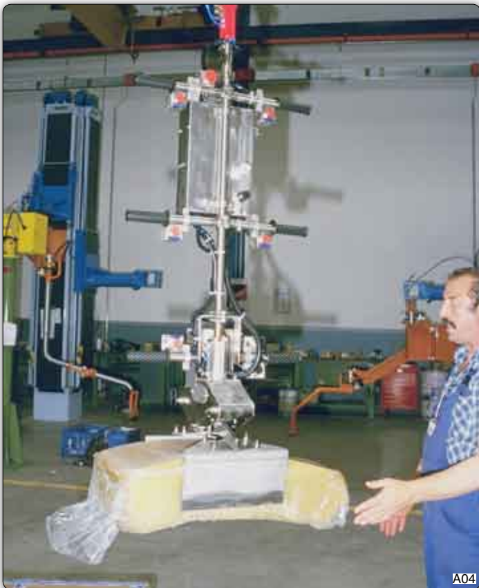
Manipulator with pneumatic jaws for handling rubber bales. The "slimline" design of the jaws allows for easy release into the bale's packaging.
