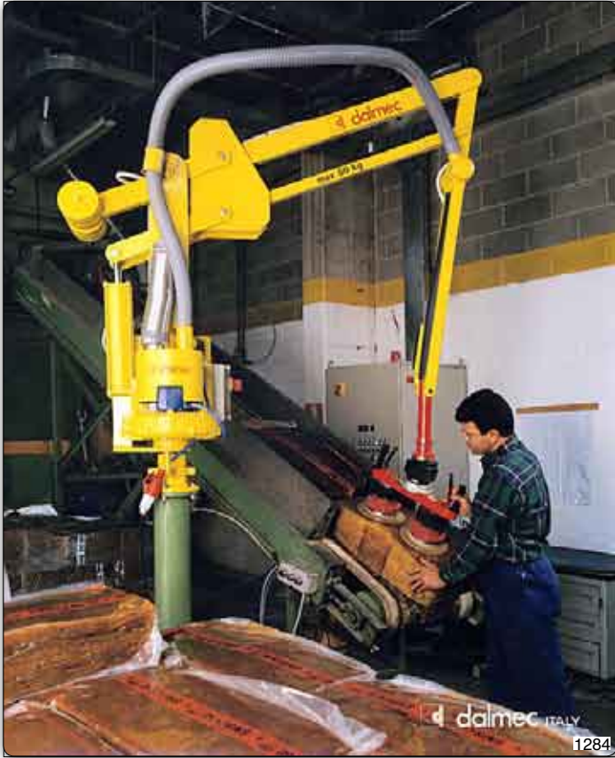
PSC type Partner manipulator, column mounted, with suction head for handling rubber bales used for a trituration plant, equipped with an "extra pull" feature to facilitate detachment of the bale from the one underneath it.
