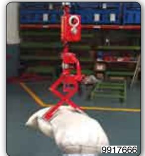
PSC type Partner manipulator, column mounted, equipped with suction head to pick bags from a pallet and to load them to a mixer.
