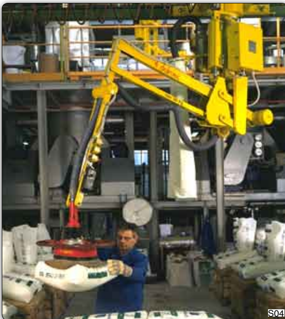
PSS type Partner manipulator, overhead trolley mounted version in Dalmecc track. The operator picks bags from various pallets in the "picking" area and deposits them to a common pallet.
