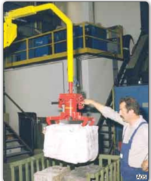
Manipulator with pneumatically actuated grippers, which hold the bale by gripping into the product itself.
