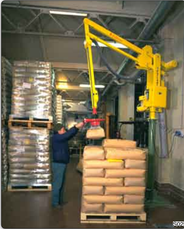
PSC type Partner manipulator, column mounted for palletization/depalletization of bags which are stacked up to about metres from floor level, fitted with lowered controls.
