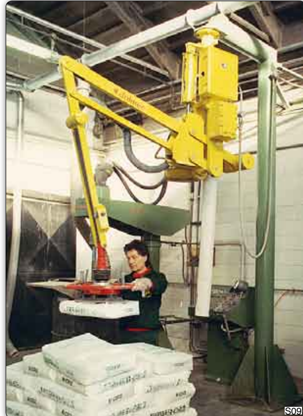
PSC type Partner manipulator, fixed version, used to move bags from a sack filler to a pallet.
