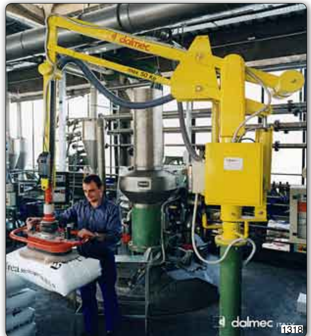
PSC type Partner manipulator, column mounted, equipped with suction head to pick bags from a pallet and loading them to a mixer.
