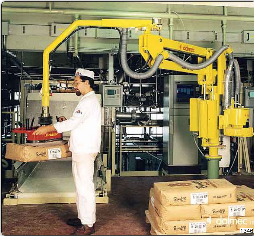
PMC type Partner manipulator, column design, special low profile unit, to enable to operate in a room with low ceiling. The equipment allows the bags to be picked from a pallet and to be loaded onto a hopper.
