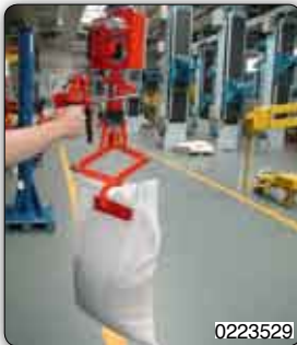
PSC type Partner manipulator, column mounted for palletization/depalletization of bags which are stacked up to about metres from floor level, fitted with lowered controls.
