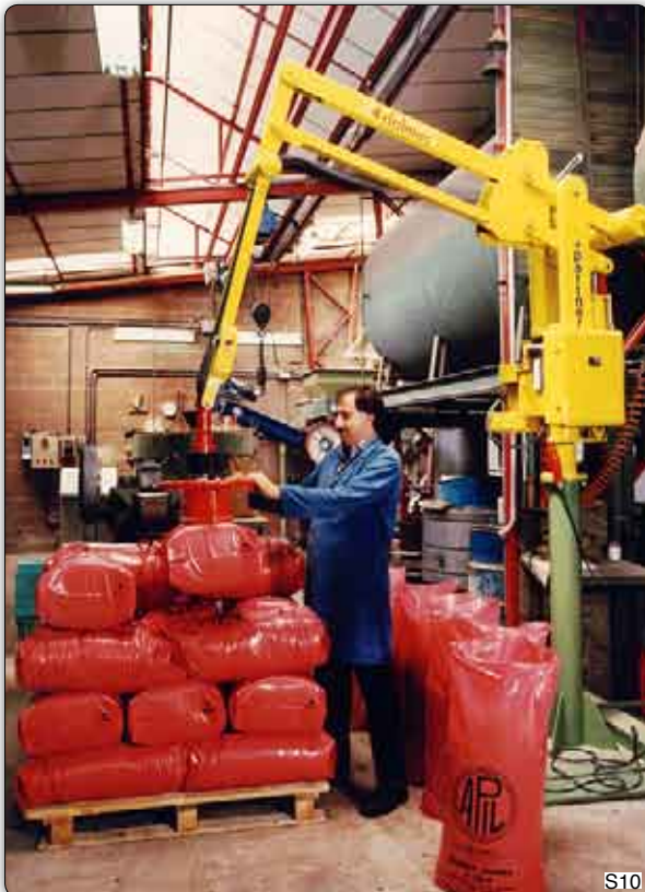
PSC type Partner manipulator, column design, overhead used to move bags from a sack filler to a pallet.
