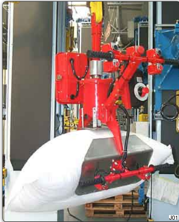
Manipulator with pneumatically actuated gripper picking system.
