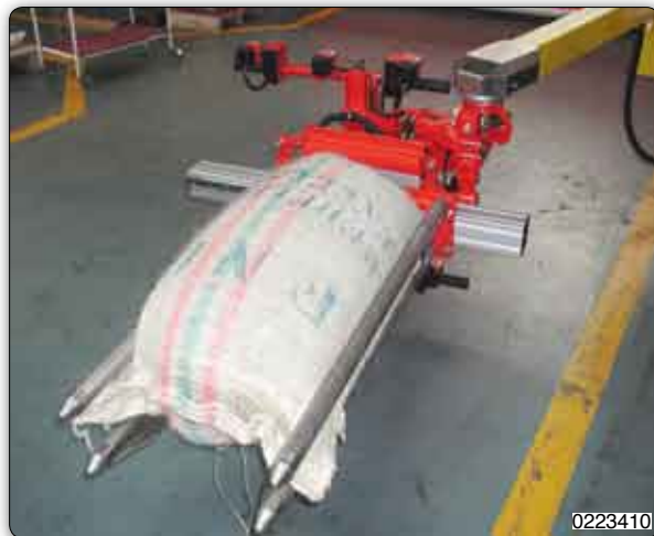
Manipulator with pneumatically actuated gripper picking system.
