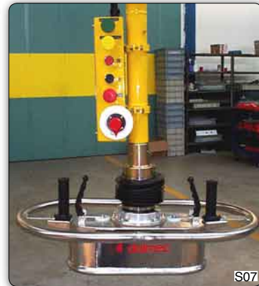
Suction device made from stainless steel.
