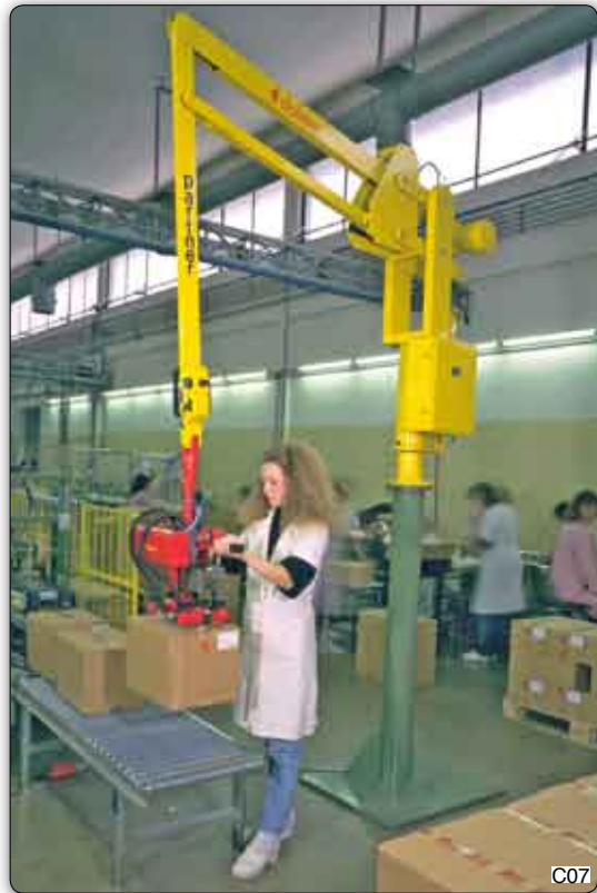
PSC type Partner manipulator, column mounted, equipped with a Venturi vacuum suction system.
