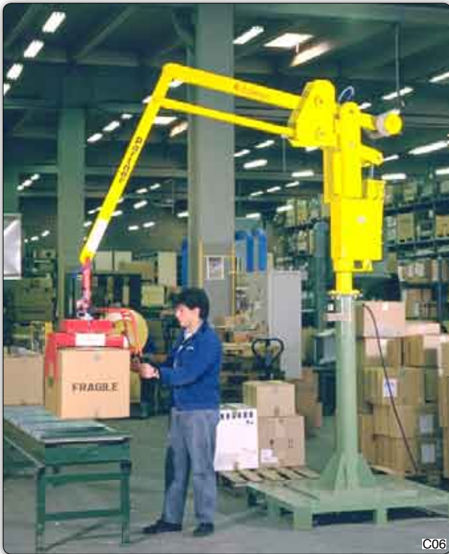
PSC type Partner manipulator, column mounted, equipped with jaws gripping system, for the picking and palletization of boxes packed with household electric appliances of various types and weights.
