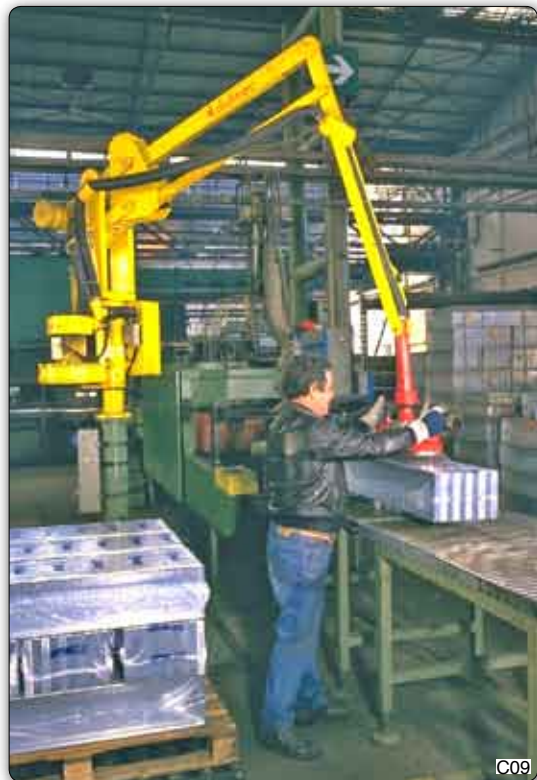
PSC type Partner manipulator, column mounted, fitted with suction cups tooling for gripping shrink-wrapped goods from a packaging line to a pallet.
