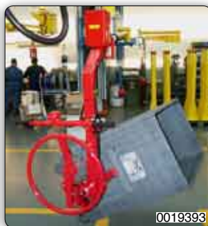
Gripping devices for handling containers of food products. In particular: - jaws tooling suitable for gripping and emptying carton boxes, containing tobacco, having different dimensions - a simple tooling for plastic boxes with manual rotation - hooks tooling made of stainless steel for handling plastic boxes - jaws stainless steel tooling for handling plastics boxes containing apples.
