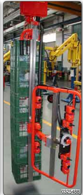
Partner Manipulator overhead trolley mounted version with pneumatic motorization, equipped with multiple adjustable hooks gripping system for handling 1 to 8 beverage crates having different dimensions.
