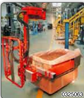
Gripping devices for handling containers of food products. In particular: - jaws tooling suitable for gripping and emptying carton boxes, containing tobacco, having different dimensions - a simple tooling for plastic boxes with manual rotation - hooks tooling made of stainless steel for handling plastic boxes - jaws stainless steel tooling for handling plastics boxes containing apples.
