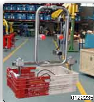
Gripping devices for handling containers of food products. In particular: - jaws tooling suitable for gripping and emptying carton boxes, containing tobacco, having different dimensions - a simple tooling for plastic boxes with manual rotation - hooks tooling made of stainless steel for handling plastic boxes - jaws stainless steel tooling for handling plastics boxes containing apples.
