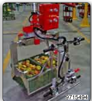
Gripping devices for handling containers of food products. In particular: - jaws tooling suitable for gripping and emptying carton boxes, containing tobacco, having different dimensions - a simple tooling for plastic boxes with manual rotation - hooks tooling made of stainless steel for handling plastic boxes - jaws stainless steel tooling for handling plastics boxes containing apples.
