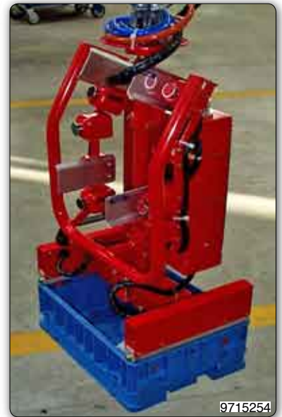
Manipulator with jaws tooling for gripping on the upper edge of the containers.
