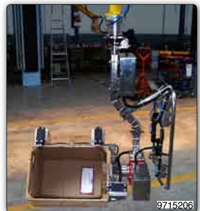
Manipulator provided with jaws tooling made of stainless steel to pick and turn cases.
