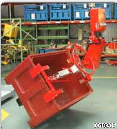
Partner PMC column mounted with pneumatic tooling for gripping, inclination and manual rotation of plastic containers having different dimensions.
