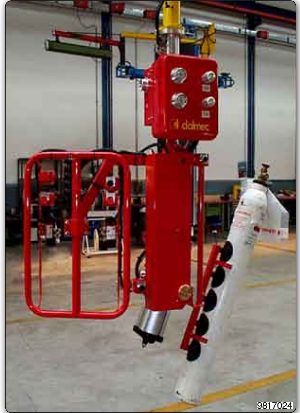
Manipulator with suction cup tooling (Venturi) for gripping and inclination of cylinders.
