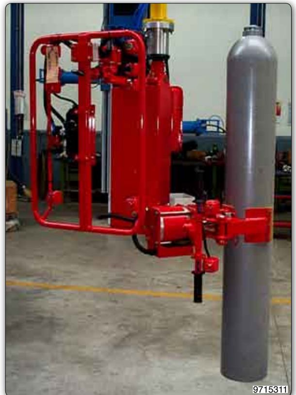
Manipulator with pneumatic tooling for gripping and inclination of cylinders having different dimensions.
