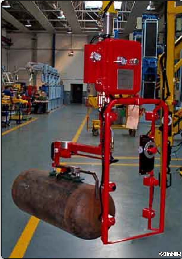
Manipulator with suction cup tooling (Venturi) for gripping and manual rotation of tanks.
