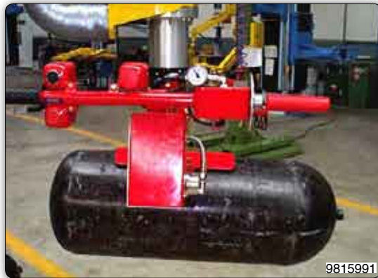
Manipulator with suction cup tooling (Venturi) for gripping and releasing the tanks into the car.
