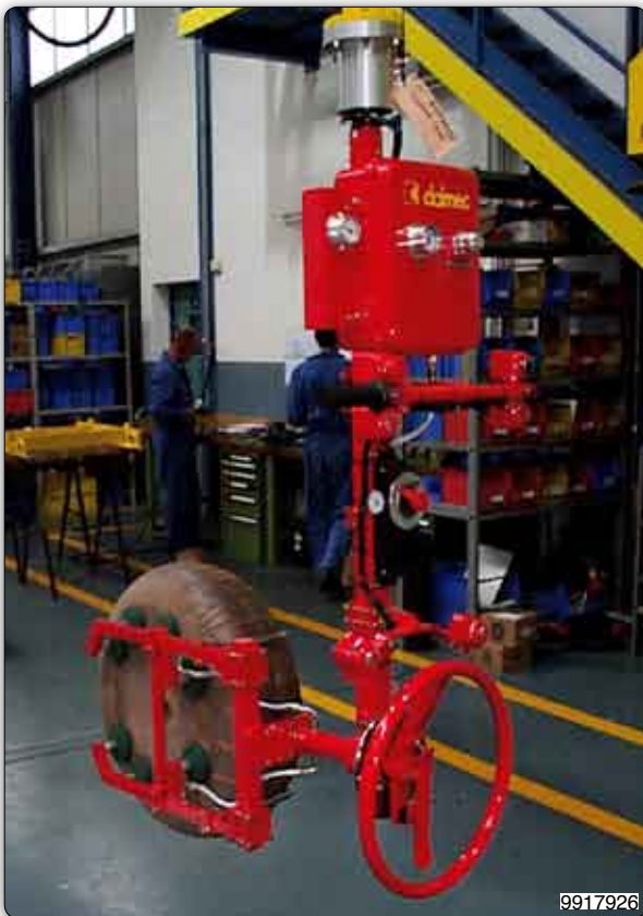
Manipulator with suction cup tooling (Venturi) for gripping and manual rotation of round tanks.
