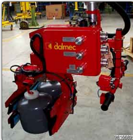
Manipulator with inflatable pads tooling for gripping one or two cylinders.
