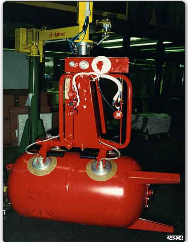
Manipulator with suction cups tooling (Venturi) for gripping and inclination of tanks.
