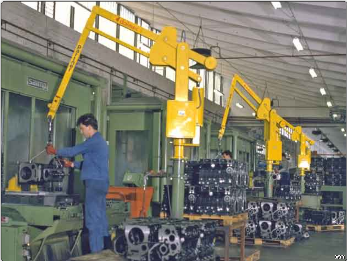
PSC type "Partner" manipulators, column mounted, used to move crankcases between various workstations.
