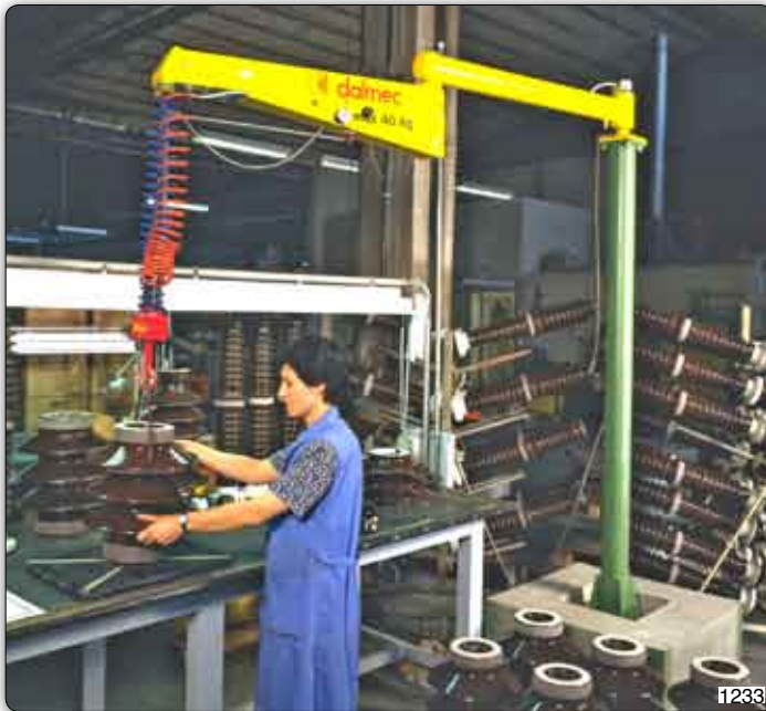
Pvc type "Posivel" manipulator, column mounted, used to move isolators.
