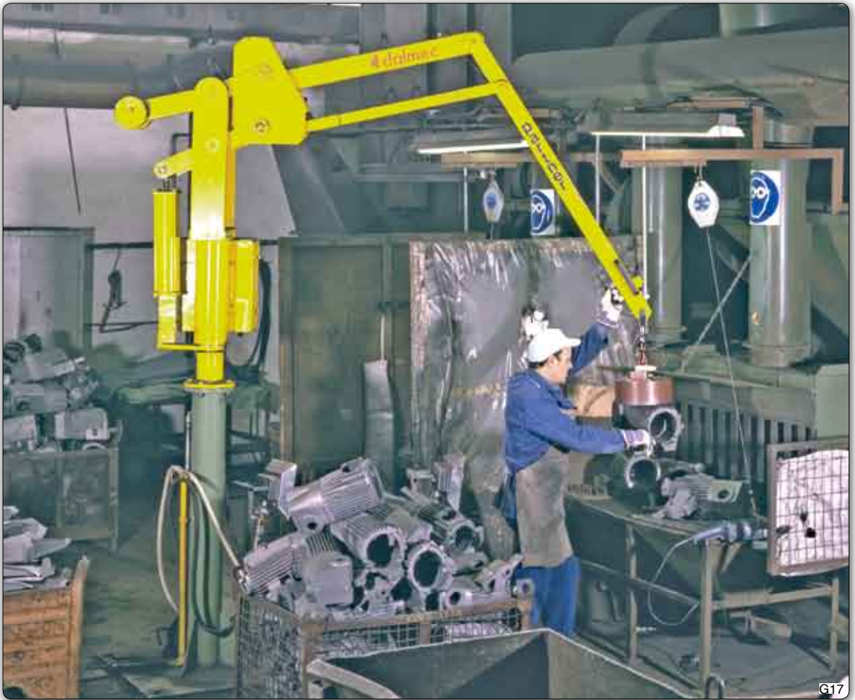
PSC type "Partner" manipulator, column mounted, designed to move stators for electric motors using a magnet supplied by the customer.
