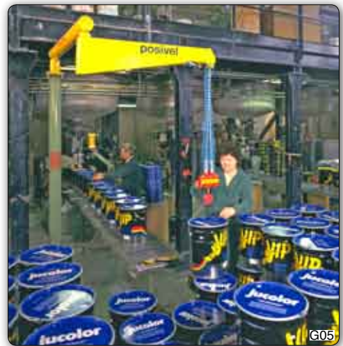
Pvc type "Posivel" manipulator, column mounted, equipped with a hook for handling drums.
