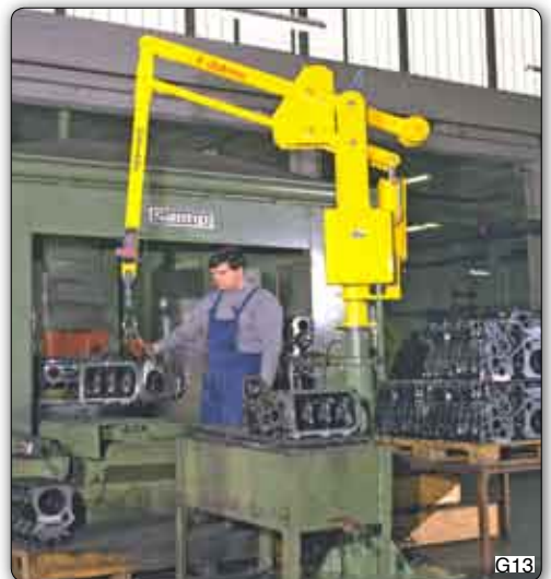
PSC type "Partner" column mounted, used for handling crankcases onto a de-greasing plant.
