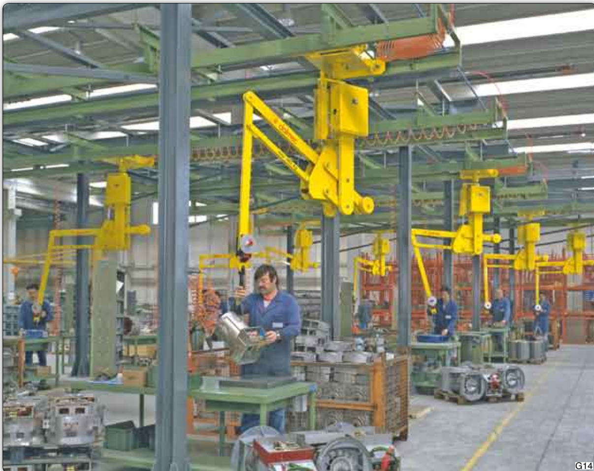
PSS type "Partner" manipulator, overhead trolley mounted machines, used to assemble electric motors. The whole system (tracking system and supporting structure) has been produced by us.
