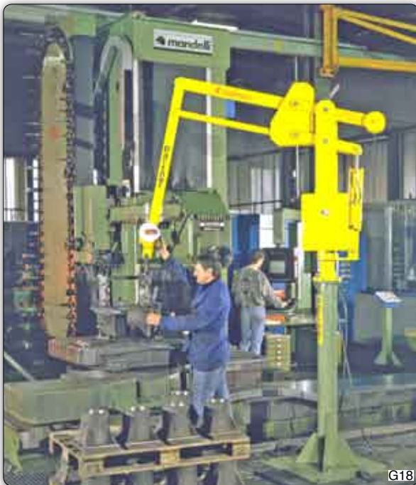
PSC "Partner" type manipulator, column mounted, used for the loading and unloading of mechanical components.
