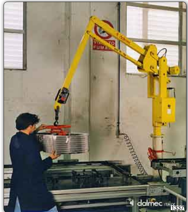
PSC type "Partner" manipulator, column mounted, designed for the loading and unloading of mechanical components.
