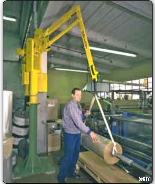
PSC type "Partner" manipulator, column mounted, used to move rolls of plastic film.
