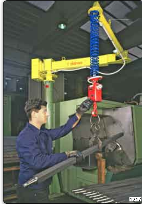
PFC type "Posifil" manipulator, column mounted version, with hook.
