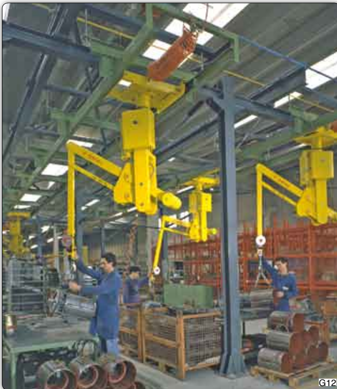
PSS type "Partner" manipulator, overhead trolley mounted, used to assemble electric motors. The tracking system and supporting structure have also been designed and manufactured by Dalmecc.
