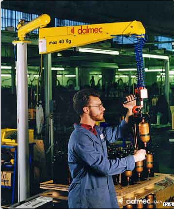
Pvc type "Posivel" manipulator, column mounted, used to move refrigeration assemblies for conditioners.
