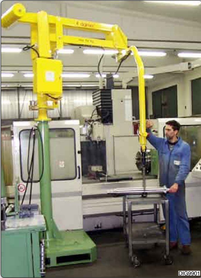
PMC type "Partner" manipulator, column mounted used for handling mechanical components.
