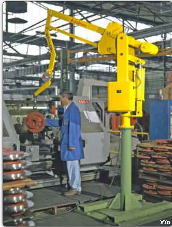
PSC type "Partner" manipulator, column mounted with gooseneck terminal arm, used to move epicycloidal spiders.
