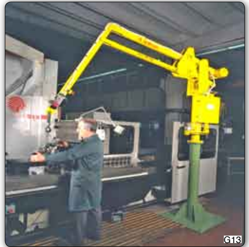
PSC type "Partner" manipulator, column mounted, designed for the loading and unloading of crankshafts from a machining centre.
