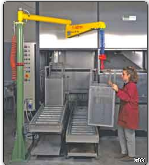
Pvc type "Posivel" manipulator, column mounted, designed to move baskets on a washing plant
