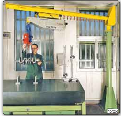
Mpc type "Minipartner" manipulator, flag-type column mounted unit, used to move crankshafts to a measuring bench.
