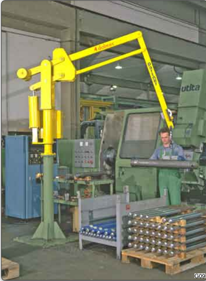
PSC type "Partner" manipulator, column mounted with extended parallelogram, used to move oleodynamic cylinders over a workstation.
