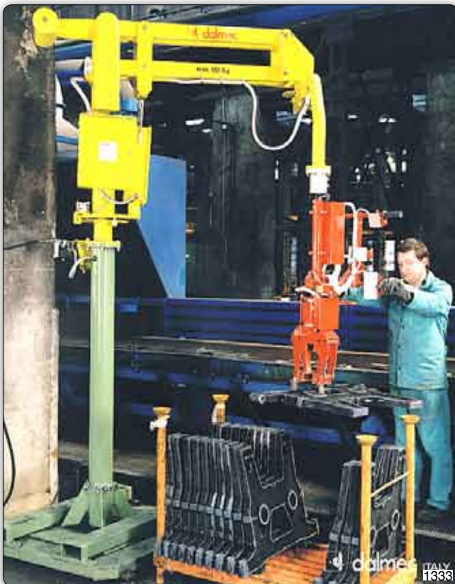
PMC type Partner manipulator, column design with special gripper equipment for taking smelted items from a conveyor belt.
