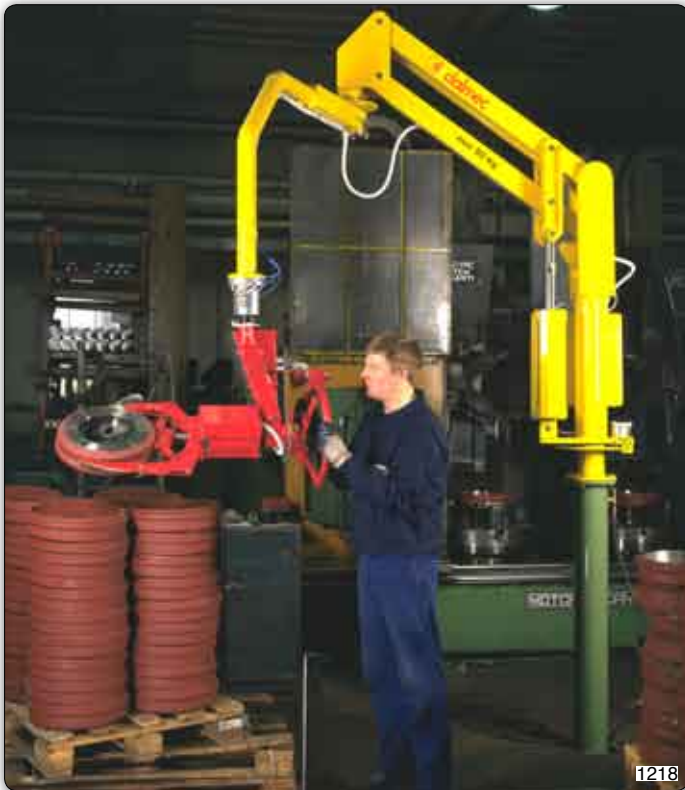
PMC type Partner manipulator, column mounted, with pneumatic tooling for picking mechanical components and manually rotating them through 180°, for use on a machining centre.
