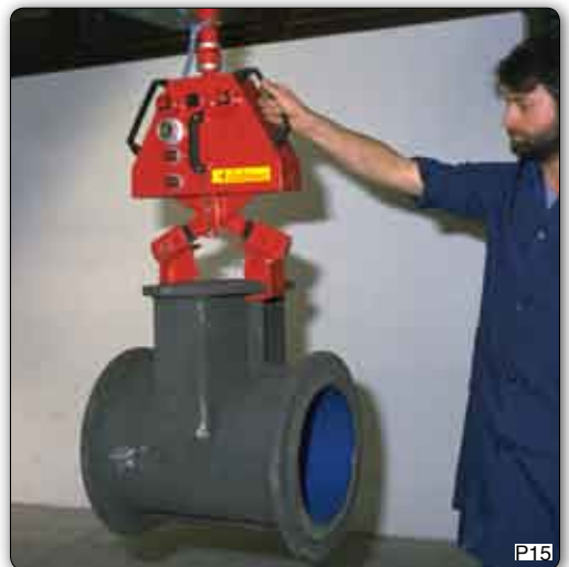
Pneumatic equipment to move valve bodies. The grippers are adjustable to allow picking of valves with different dimensions.
