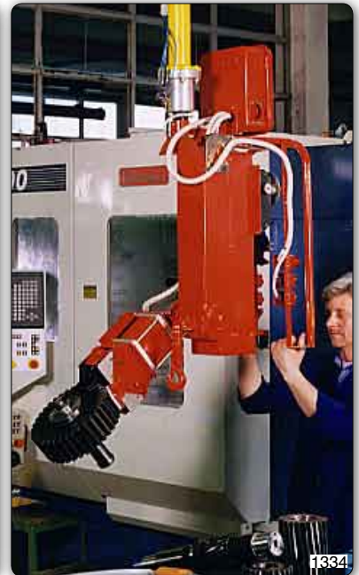
PMC type Partner manipulator, column design, with special equipment for picking, inclination and rotation of gears.
