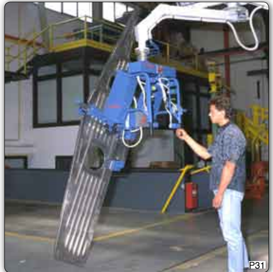
Manipulator with gripper equipment and pneumatic systems for 90° inclination and 180° rotation, for moving specific items from aircraft wings.
