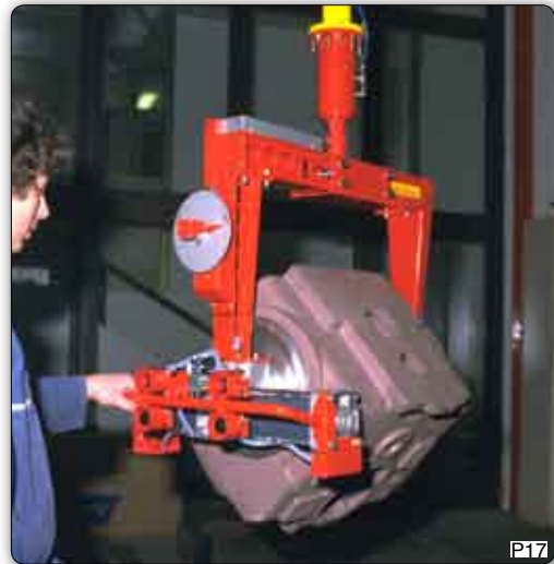
Manipulator with pneumatic equipment for taking by the two lateral holes and pneumatic rotation through 180° of reduction gear bodies, which is used for a boring machine.
