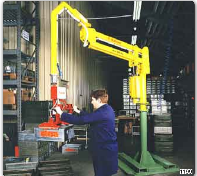
PMC type Partner manipulator, column design, equipped with gripper system to take and move metal containers.
