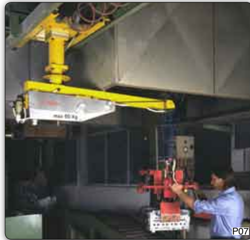
MPS type Minipartner manipulator, overhead trolley mounted running in dual track, with pneumatic tooling for the picking and placing crankcases from a roller conveyor on a pallet.
