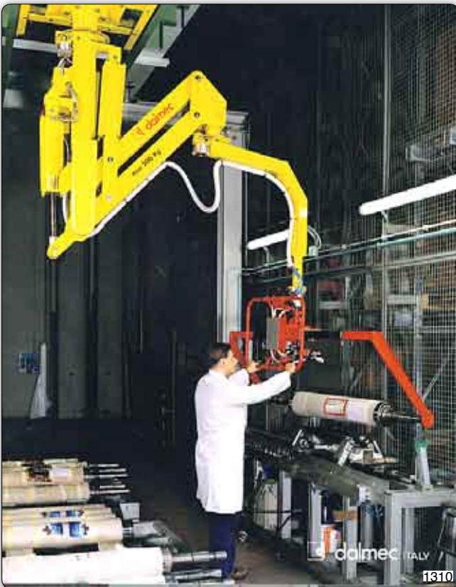
PMS type Partner manipulator, overhead trolley mounted, designed to take cylinders from the press. The equipment which is made from stirrups with shaped bushings which allow the cylinders to be taken from the pallets and put on the support of an automatic storage area, or vice versa.
