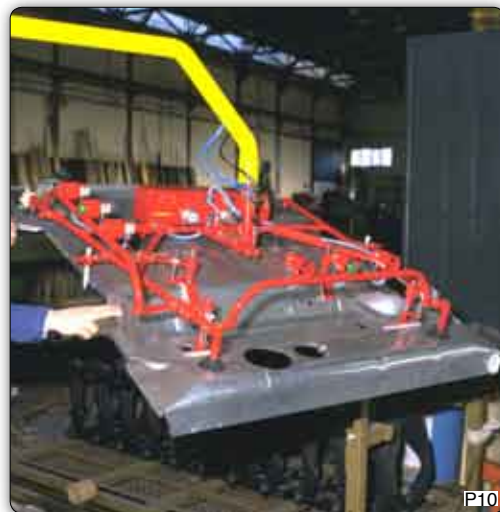
Suction tooling head used to handle motor vehicle floor pans from pallets to welding machine.
