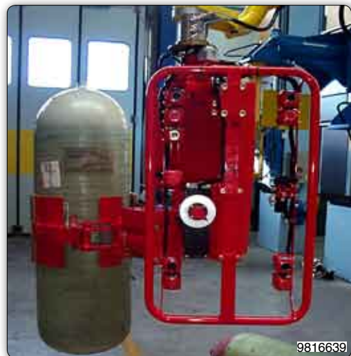
Manipulator with pneumatic gripping tool for picking and 90° pneumatic inclination of cylinders.
