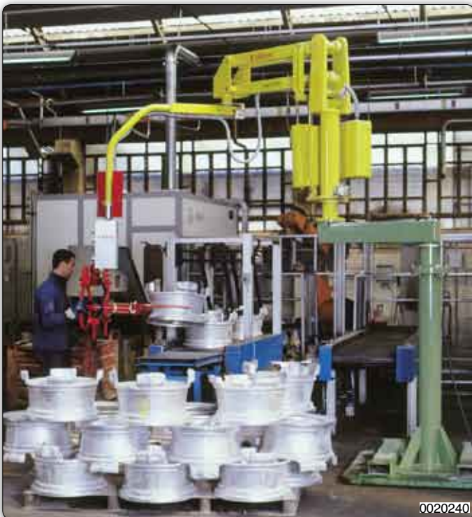
PMC type Partner, column mounted manipulator, with gripper equipment, made for taking and moving tractor rims of various sizes.
