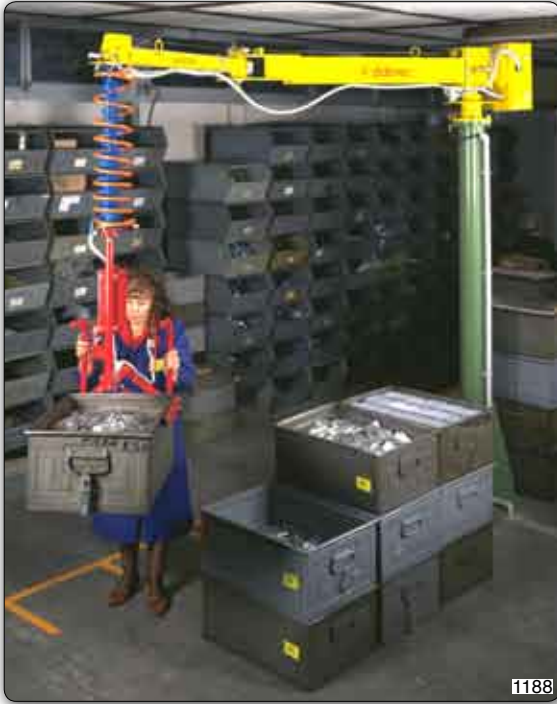
PFC type Posifil manipulator, column design, fitted with fork tooling, specially shaped to fit metal containers.
