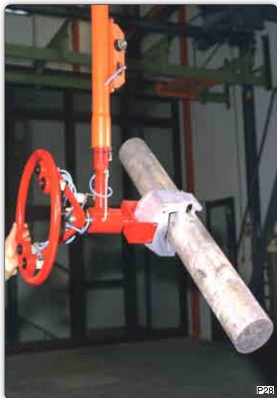
Manipulator with pneumatic gripper for moving metal bars, with 180° manual rotation.
