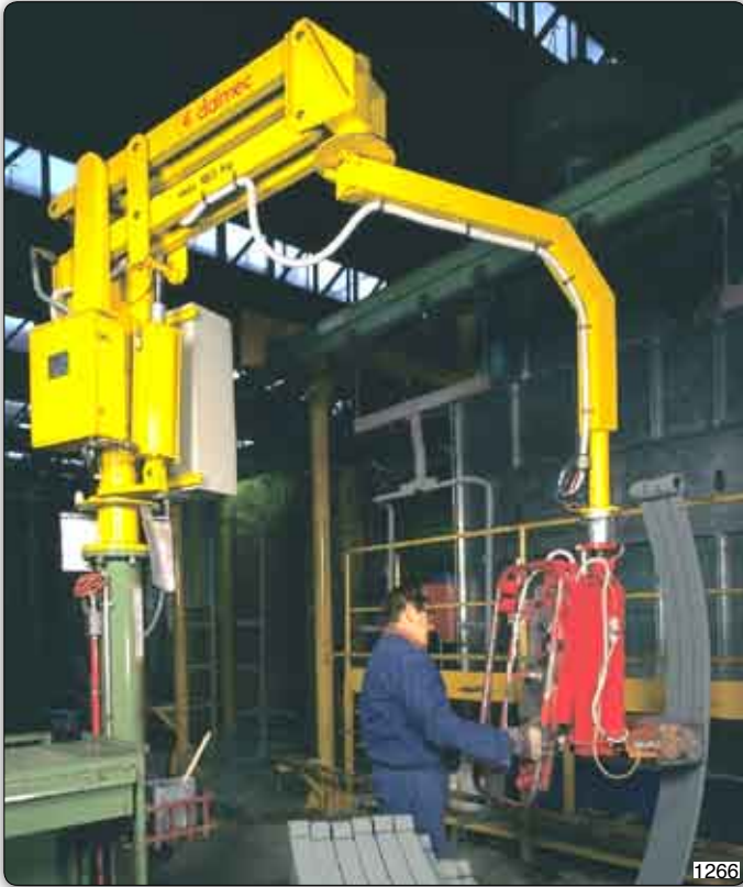
PMC type Partner manipulator, special column design, with integrated permanent electromagnets designed for taking two or three leaf springs at the same time which are placed level nearby on a pallet and, with the control of inclination up to 90°, for positioning them vertically on the balancing unit of a coating line.
