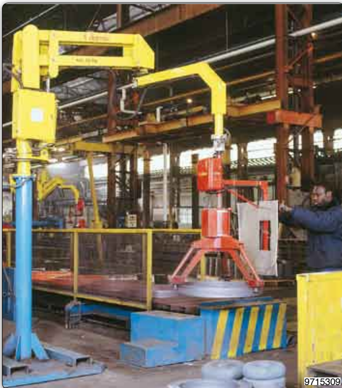
PMC type Partner manipulator, column design, with pneumatic gripper equipment, made to move mechanical parts from pallets to a vertical machine tool.
