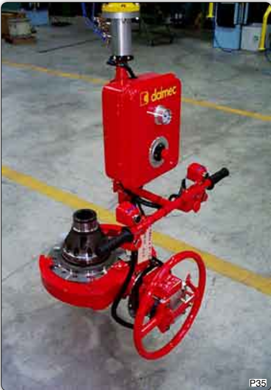
Manipulator with equipment for moving wheel hubs with 180° manual rotation.
