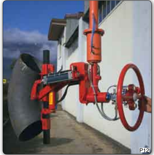
Pneumatically actuated jaws for gripping metal curved tubing, complete with pneumatic 90° inclination system and manual rotation through 180°.
