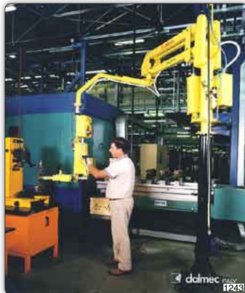
PMC type Partner manipulator, column mounted, equipped with pneumatic tooling for the picking and rotation of mechanical components.
