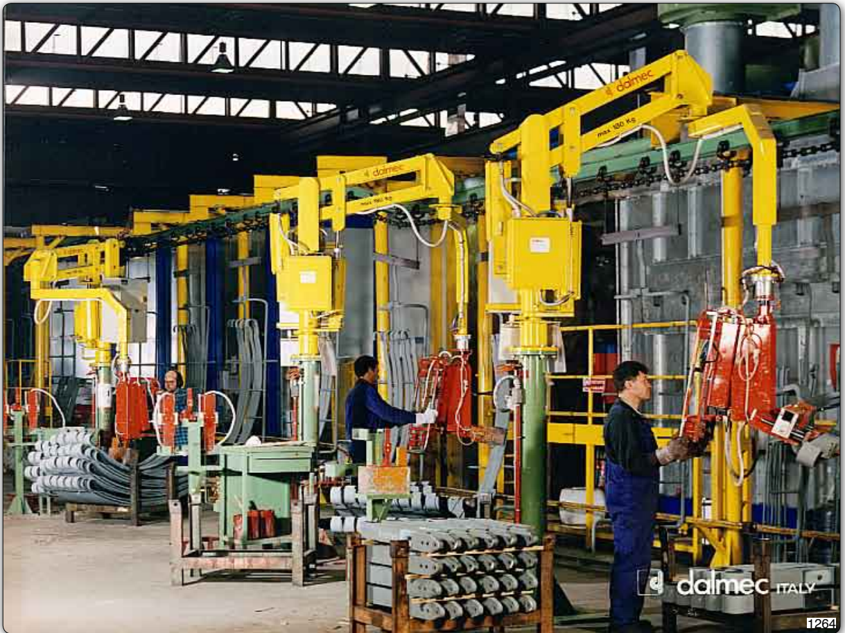
PMC type Partner manipulator, column design, equipped for loading and unloading of assembled leaf springs from a coating plant. The Manipulators have been given two types of picking equipment, which may be interchanged quickly: one uses a permanent magnet with electronic control and the other uses grippers.
