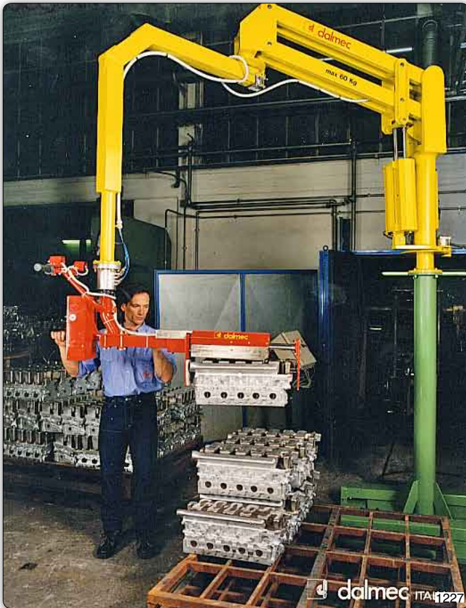
PMC type Partner manipulator, column mounted version, used for the handling of crankcase sets..
