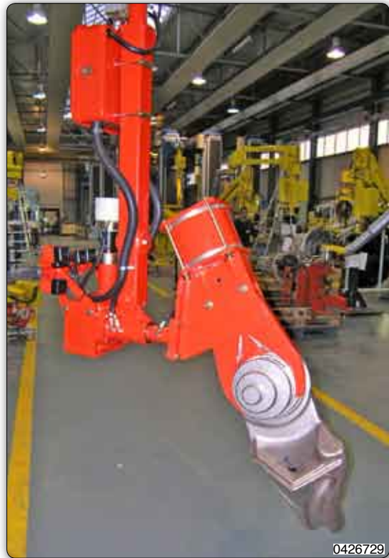
Pinch jaws tooling for the gripping and pneumatic rotation of milling machines parts having different forms and weights.
