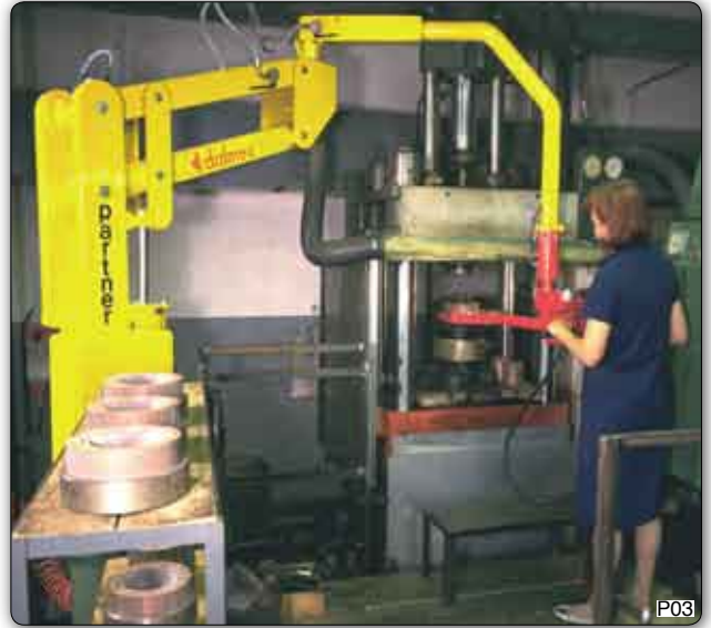
PMC type Partner manipulator, low profile column unit for operating in an area with low ceiling height. The unit is equipped with pneumatic grippers for handling electrical collectors, and enables the operator to handle them in a off-set position.
