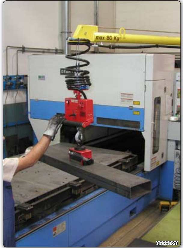
Manipulator with bipolar permanent magnet with manual action, equipped with anti-release safety device which prevents the tooling from releasing the load before it is correctly in place.
