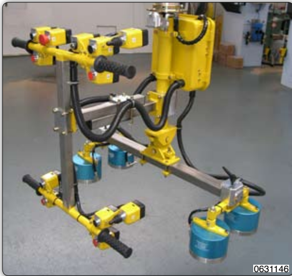
Manipulator equipped with multipolar magnets pneumatically operated for gripping and lifting steel sheets. The distance between centres of the magnets is manually adjustable.
