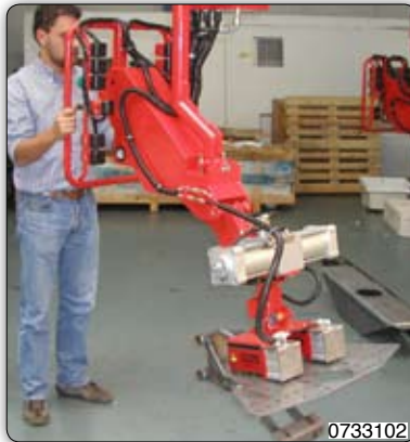
Manipulator with multipolar permanent magnets pneumatically operated, for gripping steel products with inclination up to 90° and rotation up to 180°.
