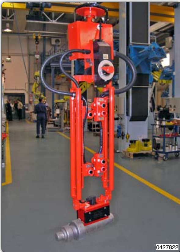
Manipulator with electropermanent magnet and pantograph handles to facilitate the positioning of the magnet on mechanical parts placed higgledy-piggledy in a container.
