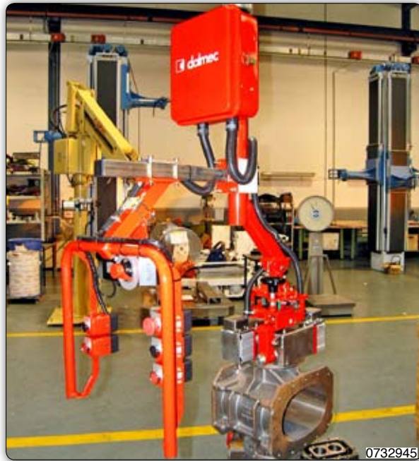
Manipulator equipped with multipolar permanent magnets pneumatically operated, for gripping and lifting steel products.
