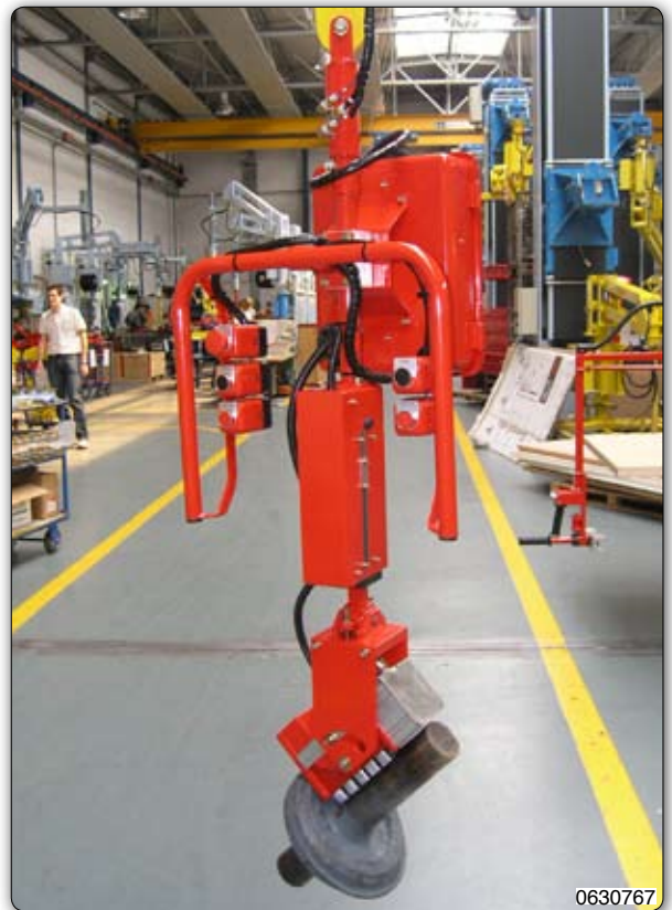
Manipulator with multipolar permanent magnet with pneumatic action, for gripping and lifting mechanical parts placed jumbled in a container.
