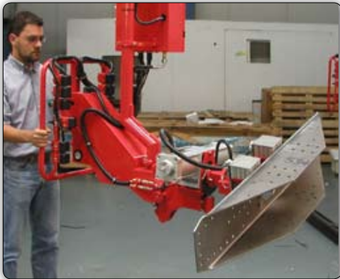
Manipulator with multipolar permanent magnets pneumatically operated for gripping and lifting steel strap rolls. The distance between centres of the magnets is manually adjustable.
