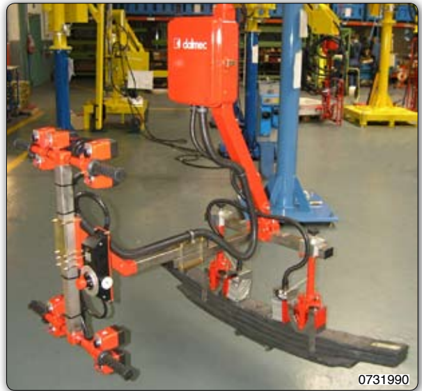
Manipulator equipped with multipolar magnets pneumatically operated for gripping and lifting leaf springs. The position of the magnets may be adjustable manually.
