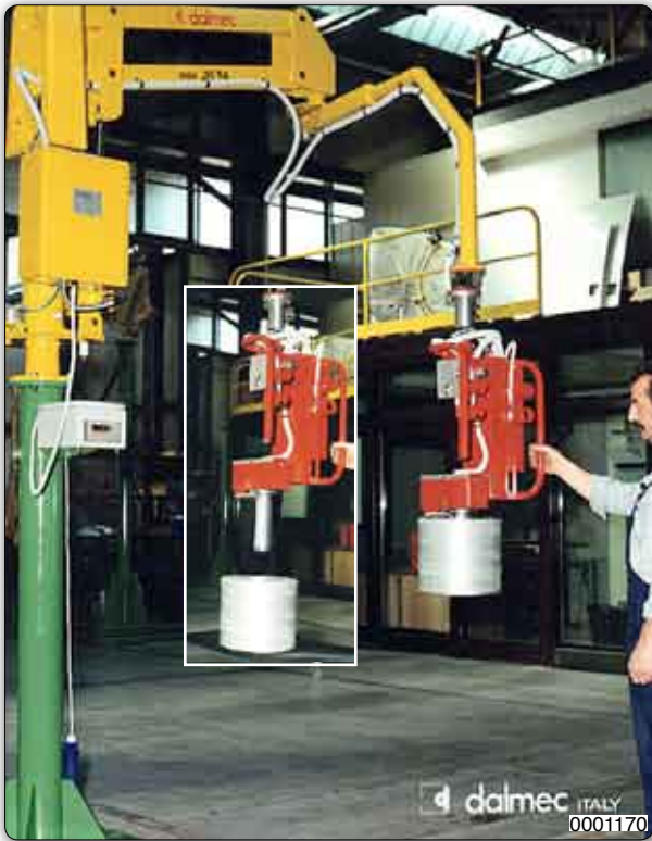
PMC type Partner manipulator, column mounted, equipped with an expanding mandrel for handling and 90° inclination of reels. The manipulator has a load cell for checking the weight of the reels.
