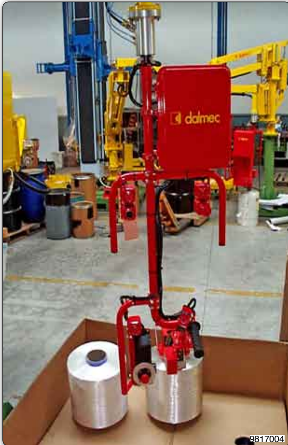
Manipulator with pneumatic expansion equipment for handling reels, fitted with manual rotation, to index the reel from the horizontal to the vertical.
