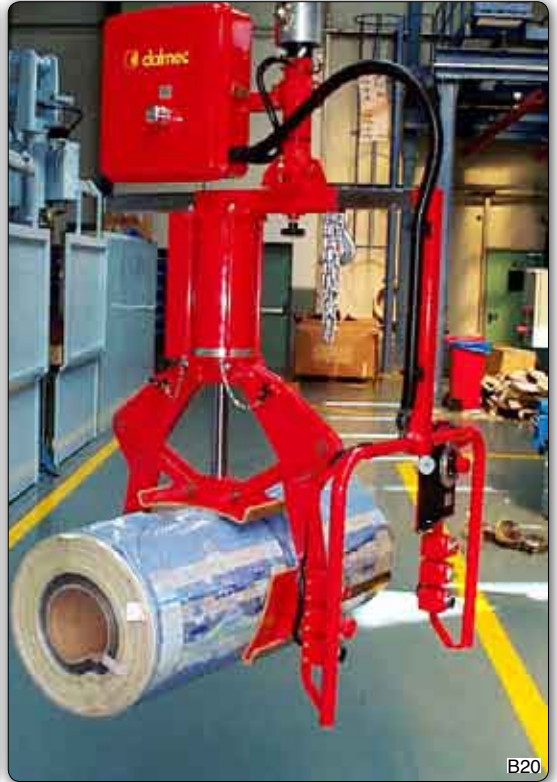
Manipulator fitted with pneumatic grippers for handling reels about their outside diameter.
