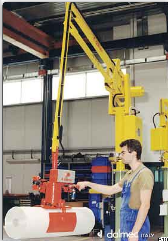
PSC column-type Partner, with pneumatic gripping jaws for handling rolls about their external diameter.
