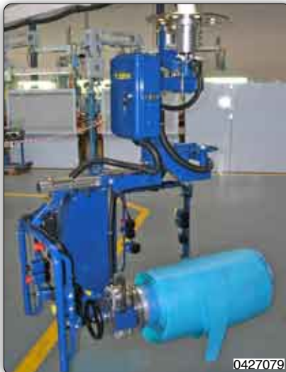
Manipulator with expanding mandrel for picking, inclination and manual rotation of reels.
