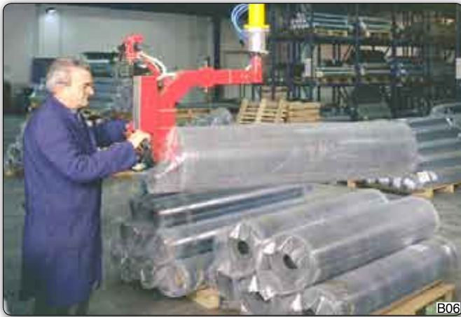
Manipulator with tooling for handling rolls of rubber from a packaging line to a pallet, made up of a pin which is inserted into the core of the roll.
