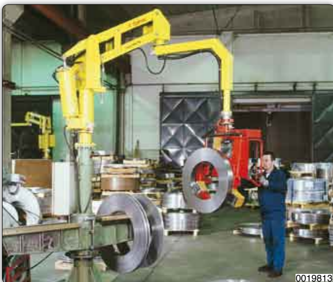
PMC type Partner manipulator, column version, equipped with a magnet for gripping and 90° inclination of rolls of metallic banding.
