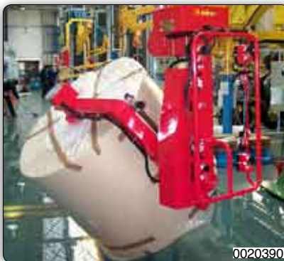
Expanding mandrel for the pneumatic rotation of reels.
