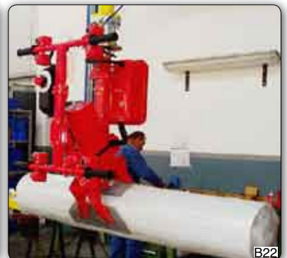
Manipulator with pneumatic gripping jaws for the easy picking of stacked reels about their external diameter.
