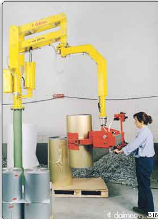
PMC type Partner manipulator, column mounted, with gripper tooling, for handling reels about their external diameter, with pneumatically assisted rotation through +/- 90°.
