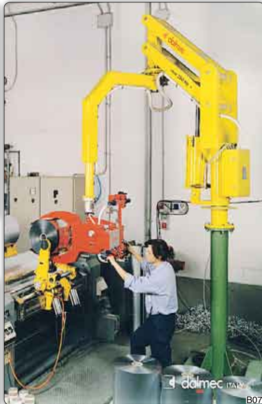
PMC type Partner manipulator, column design, provided with gripper tooling for picking and unwinding reels of plastic film from a cutting machine. With pneumatically assisted rotation through an angle of 90°, the individual reels are then positioned vertically on the pallet.
