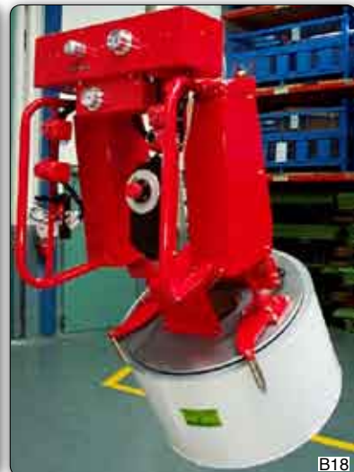
Manipulator with "Venturi" vacuum suction ring and 90° pneumatic inclination.
