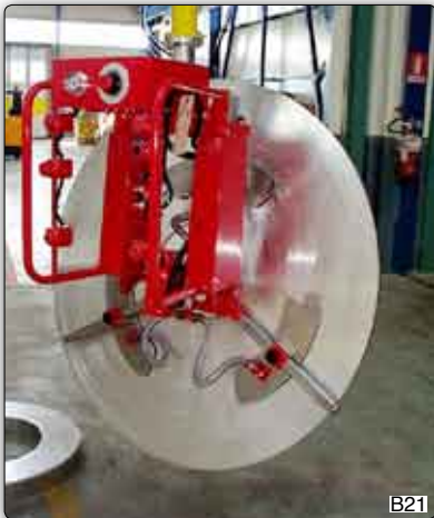
Manipulator with manually adjustable suction cups tooling for gripping and 90° inclination of rolls of metallic banding.
