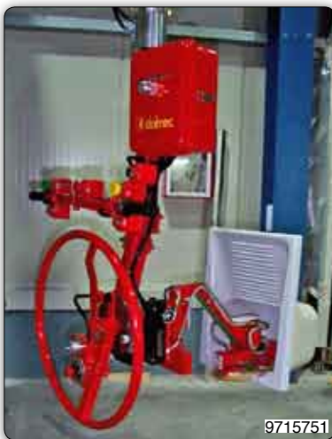
Manipulator with suction cups tooling (Venturi) for gripping and manual rotation of sinks.
