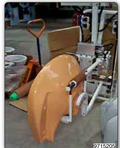
Manipulator with adjustable forks type tooling for gripping and handling sinks.
