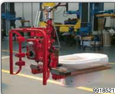
Adjustable suction cups toolings for handling WC.
