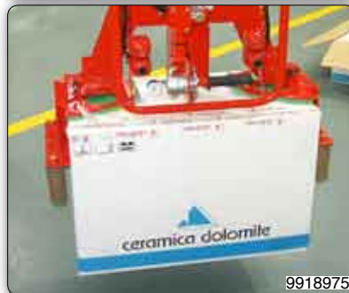
Manipulator with jaws tooling for gripping sanitary, their releasing into the cartons, gripping the packaged boxes and their pallettization.
