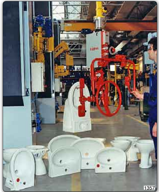
Manipulator with suction cup tooling for gripping and manual rotation of WC.
