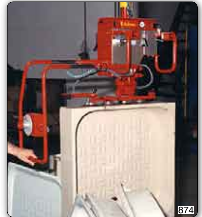
PMF Partner Manipulator, fixed overhead, with suction cups tooling (Venturi) for gripping and manual rotation of shower plates.
