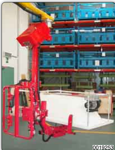
Suction cups (Venturi) Manipulator for gripping and rotation of bathtubs.
