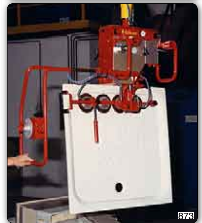
Manipulator with suction cups tooling (Venturi) for gripping shower plates.
