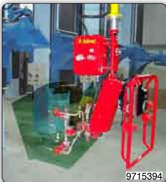
Adjustable suction cups tooling for handling and 90° pneumatic inclination of glass sheets.
