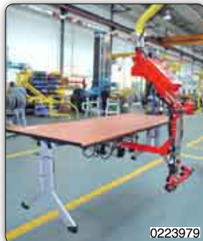
Vacuum suction systems and pneumatic or manual inclination/rotation for handling different types of products.
