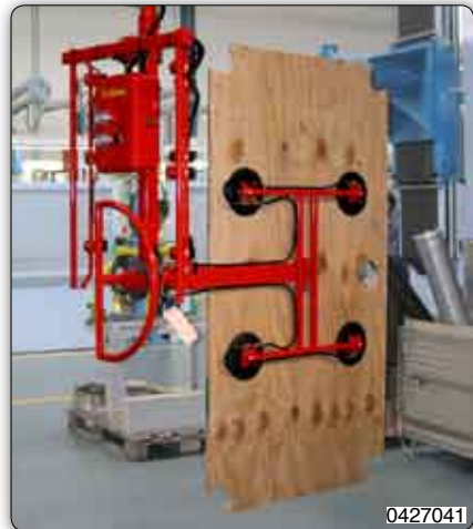
Suction cups tooling for handling wooden panels with manual rotation.
