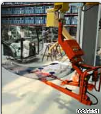
Vacuum suction system and manual inclination for handling glasses.
