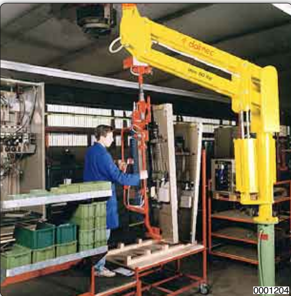
PMC type Partner manipulator, column mounted equipped with jaws tooling for gripping and handling doors of drink machines.
