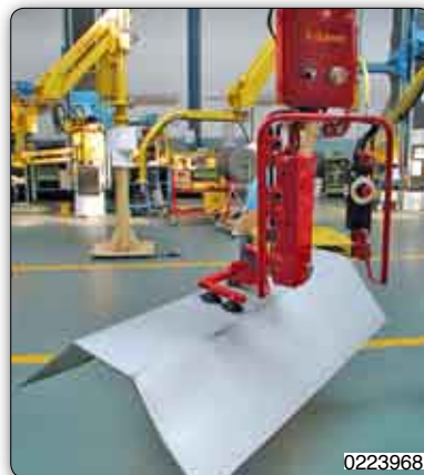
Suction cups toolings for handling sheets with manual or pneumatic rotation.
