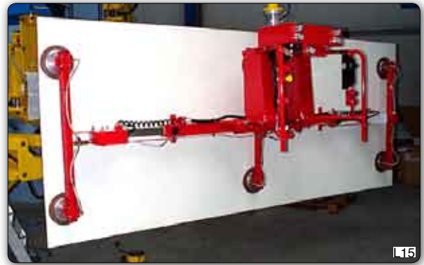
Manipulator with suction tooling designed for the picking and pneumatic inclination by 90° of sheets of laminated plastic. Positioning of the individual suction cups may be changed manually in relation to the dimensions of the panels to be moved. Vacuum is generated by a venturi ejector which is fitted on the outside of the tooling head.
