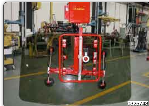
Manipulator with vacuum suction system and manual rotation for handling windscreens.
