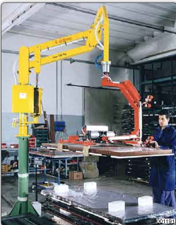
PMC type Partner manipulator, column mounted, fitted with two self-centering pairs of grippers, for picking reinforced doors and then rotating them through 180°.
