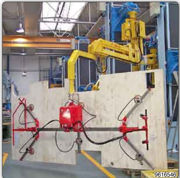
PMF type Partner manipulator, fixed overhead unit, equipped with suction tooling for the handling and pneumatic inclination through an angle of 90° of panels for camper vans. The position of each suction cup may be adjusted manually.
