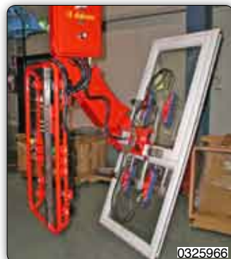
Adjustable suction cups tooling pneumatic inclination for handling door and window frames.
