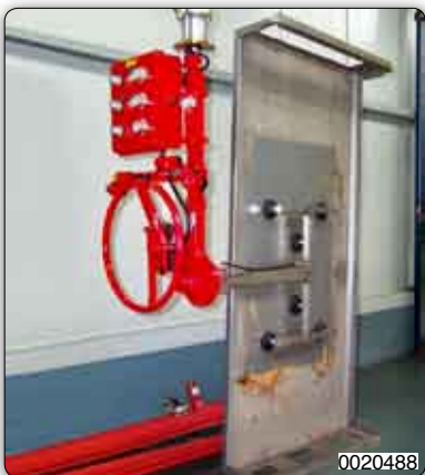
Suction cups toolings for handling sheets with manual or pneumatic rotation.
