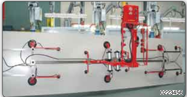
PMS type Partner manipulator, overhead trolley mounted with motorised pneumatic drive, fitted with adjustable suction cups tooling for handling and inclination of big panels.
