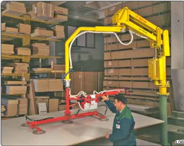
PMC type Partner manipulator, column mounted, fitted with suction head for picking a panel from a pallet and then for placing it onto a framing machine following shaving.
