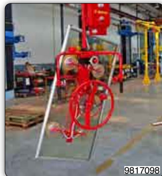
Suction cups tooling for handling and 360° manual rotation of panes of glass.
