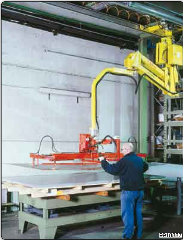
PMS type Partner manipulator, overhead trolley mounted, equipped with a suction system for picking sheets of stainless steel, picking them level from a pallet, moving them and depositing the same on another adjacent pallet. The servo-assisted inclination allows the operator to make a visual inspection of the sheet.
