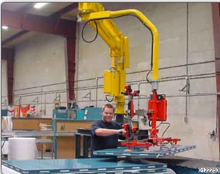
PMC type Partner manipulator, column mounted, fitted with adjustable suction cups tooling for handling panels.
