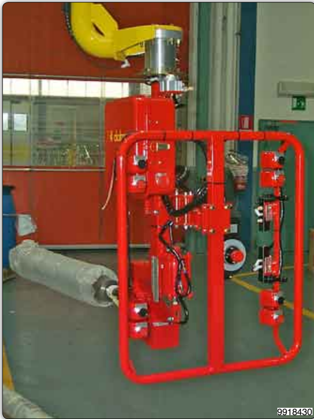
Manipulator with pneumatic tooling for gripping and handling shafts.
