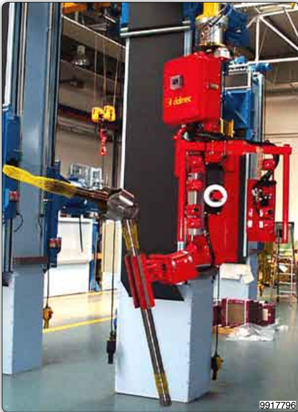
Manipulator with pneumatic tooling for gripping, inclination and rotation of transmission shafts.
