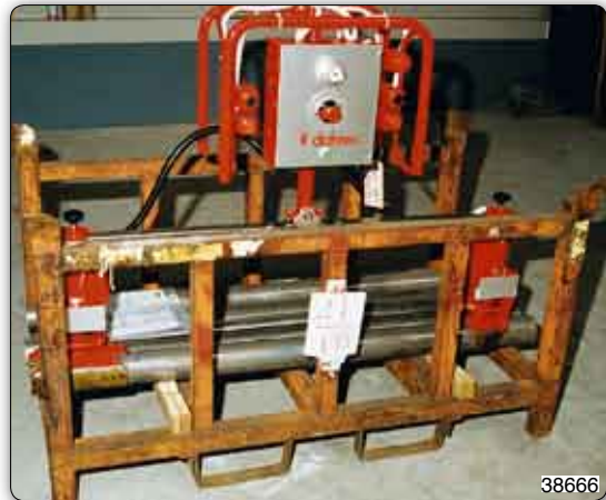
Manipulator with double gripping head tooling for gripping and handling transmission shafts.
