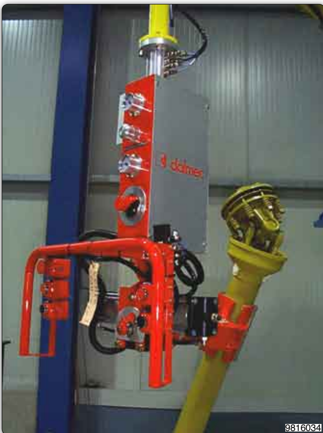
Manipulator with pneumatic tooling for gripping and rotation of transmission shafts.
