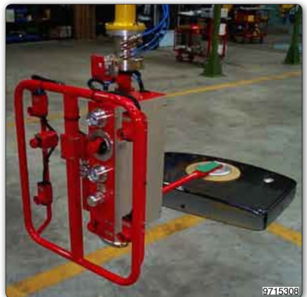
Manipulator with suction cups tooling for gripping and 90° inclination of glasses for TV tubes.
