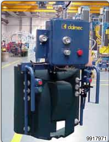
Manipulator with suction cups tooling for gripping and handling TV.
