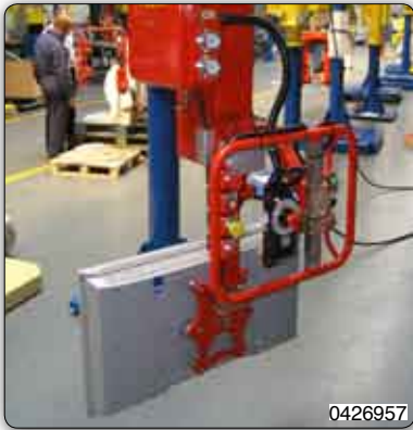
Manipulator with suction cups tooling for gripping and handling TV LCD.
