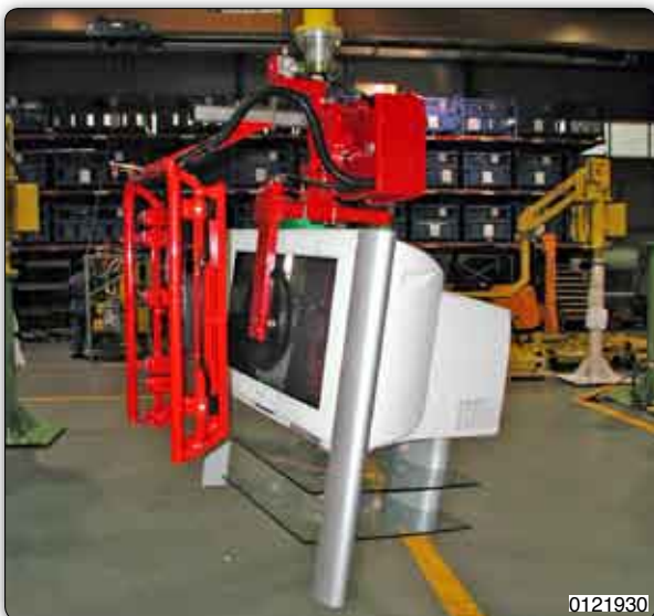
Manipulator with suction cups tooling for gripping and handling TV.
