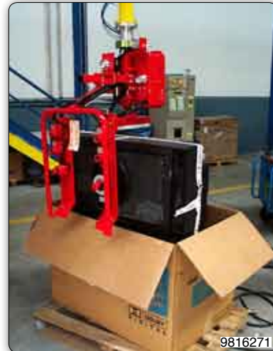
Manipulator with suction cups tooling for gripping on the screen, handling and placing into the appropriate TV packing.
