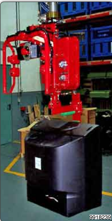
Manipulator with suction cups tooling for gripping on the screen, handling and placing into the appropriate TV packing.
