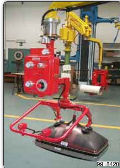
Manipulator with suction cups tooling (Venturi) for gripping and handling of TV tubes on the cone.
