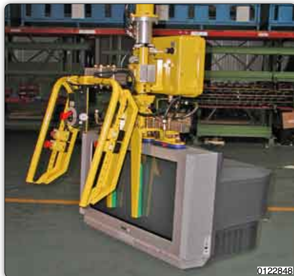
Manipulator with suction cups tooling for gripping on the screen, handling and placing into the appropriate TV packing.
