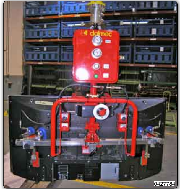
Manipulator with suction cups tooling for gripping and handling TV LCD.
