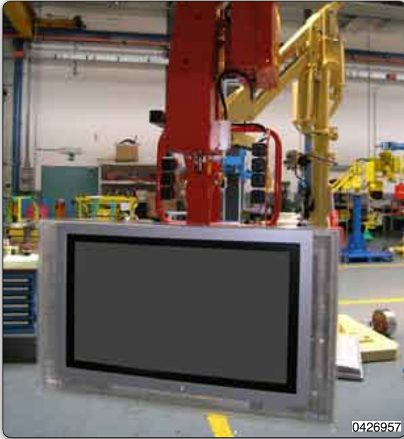
Manipulator with suction cups tooling for gripping and handling TV LCD.
