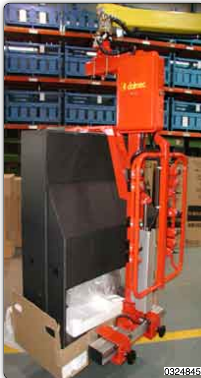
Manipulator with forks tooling for handling packaged televisions.
