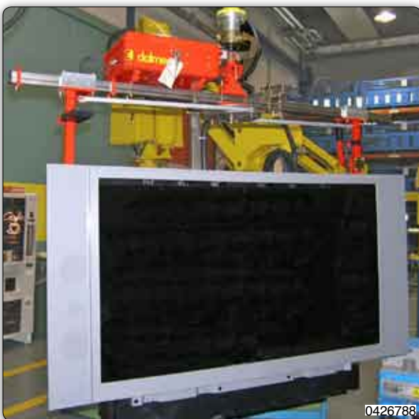
Manipulator with suction cups tooling for gripping and handling TV LCD.
