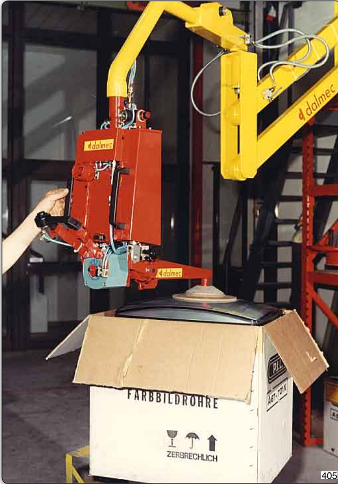
Manipulators with suction cup tooling (Venturi) for gripping, inclination and rotation of TV tubes.
