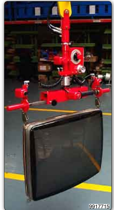
Manipulator with adjustable hooks tooling for gripping the TV tube on the supports.
