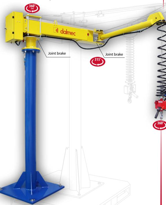
POSIPLUS PP, is a double cable manipulator with high load capacities, it is able to handle loads up to 200 kg and reaches working radii up to 4500 mm. The gripping tool is connected to the balancing group through two independent steel cables to ensure maximum safety. The particular double-arm structure with intermediate joint makes it easy to operate within the entire working area. Specific brakes mounted on the main joints guarantee control of drift movements.
